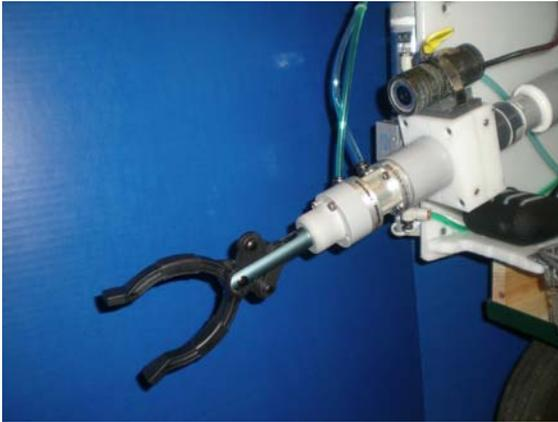
Figure 9 - Multi Axis Manipulator Arm
