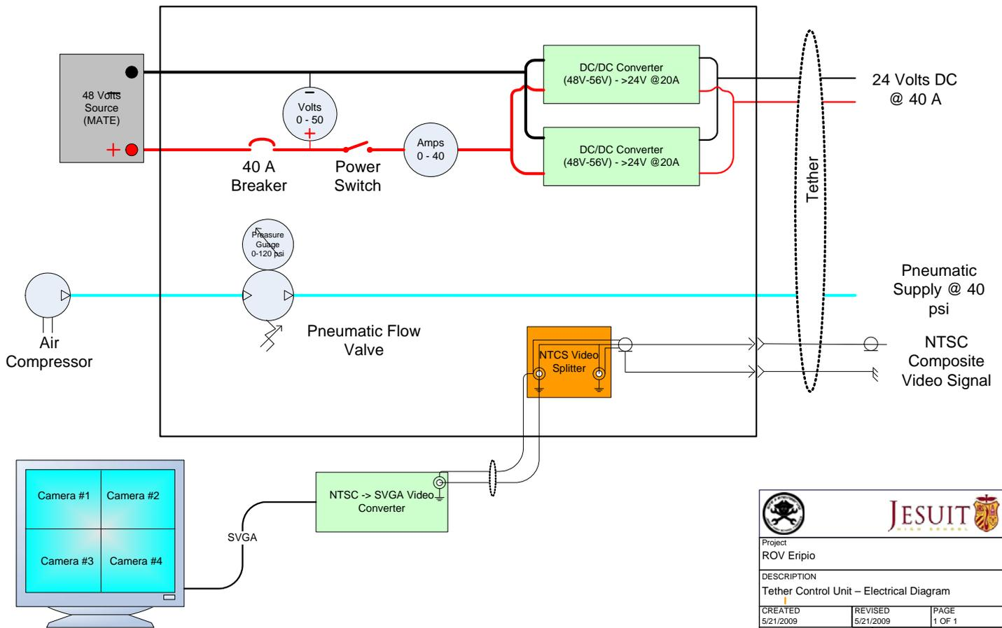
Figure 5 - Tether Control Unit Electrical Diagram
