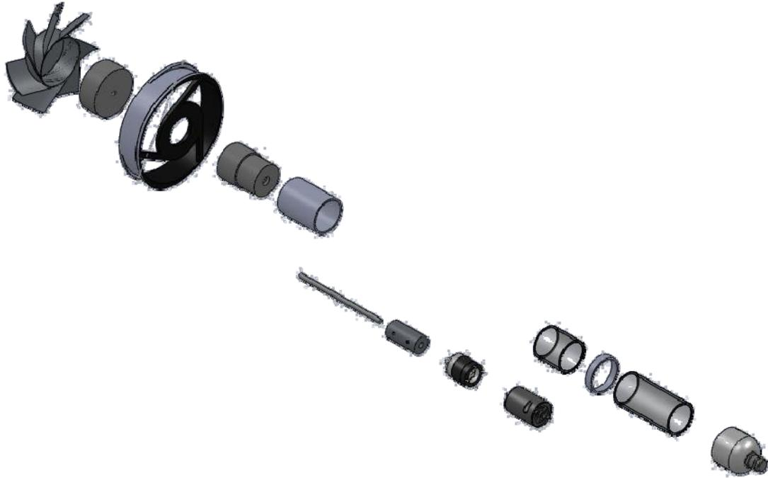
Figure 1 - J-2 Thruster Exploded CAD Rendering
