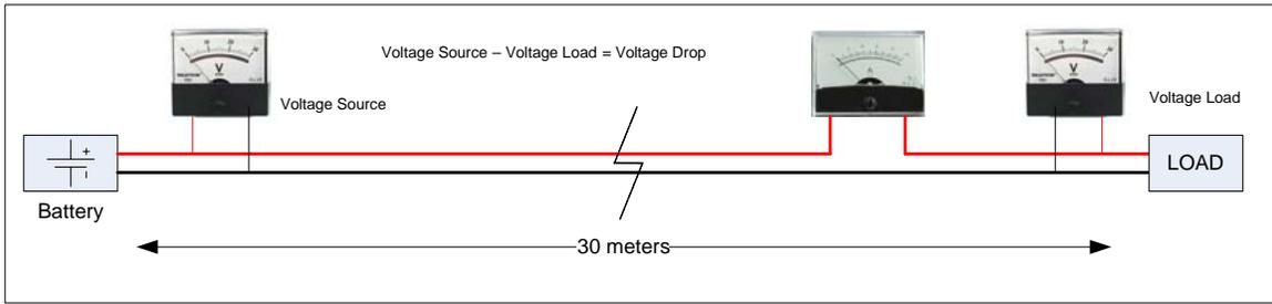
Figure 13 – Measuring voltage drop over length of tether
