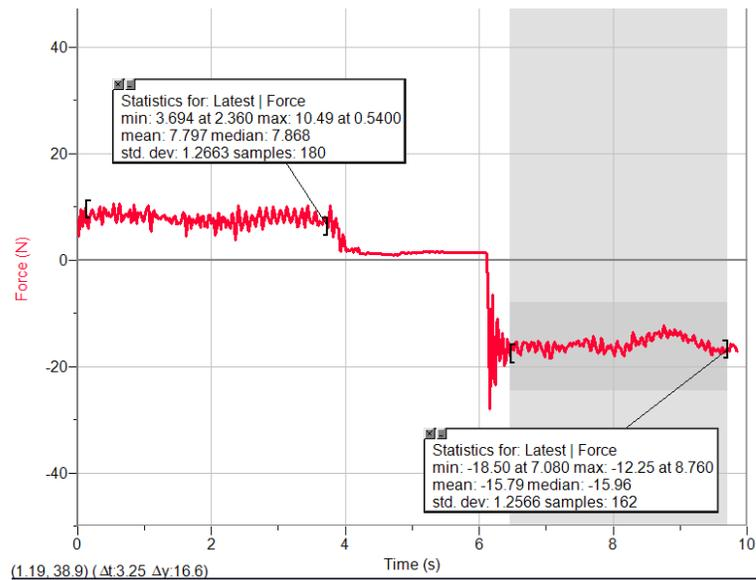
Figure 2 – J-2 Thruster Thrust Profile
