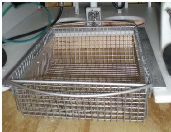
Figure 12 - Retrieval Basket Payload Attachment
