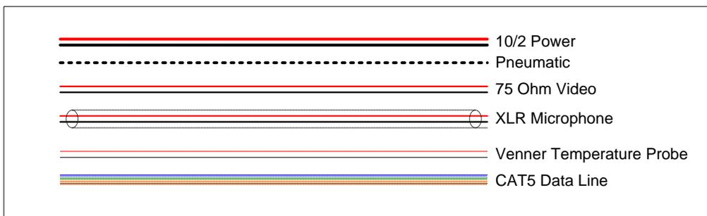
Figure 4 - ROV Tether Components
