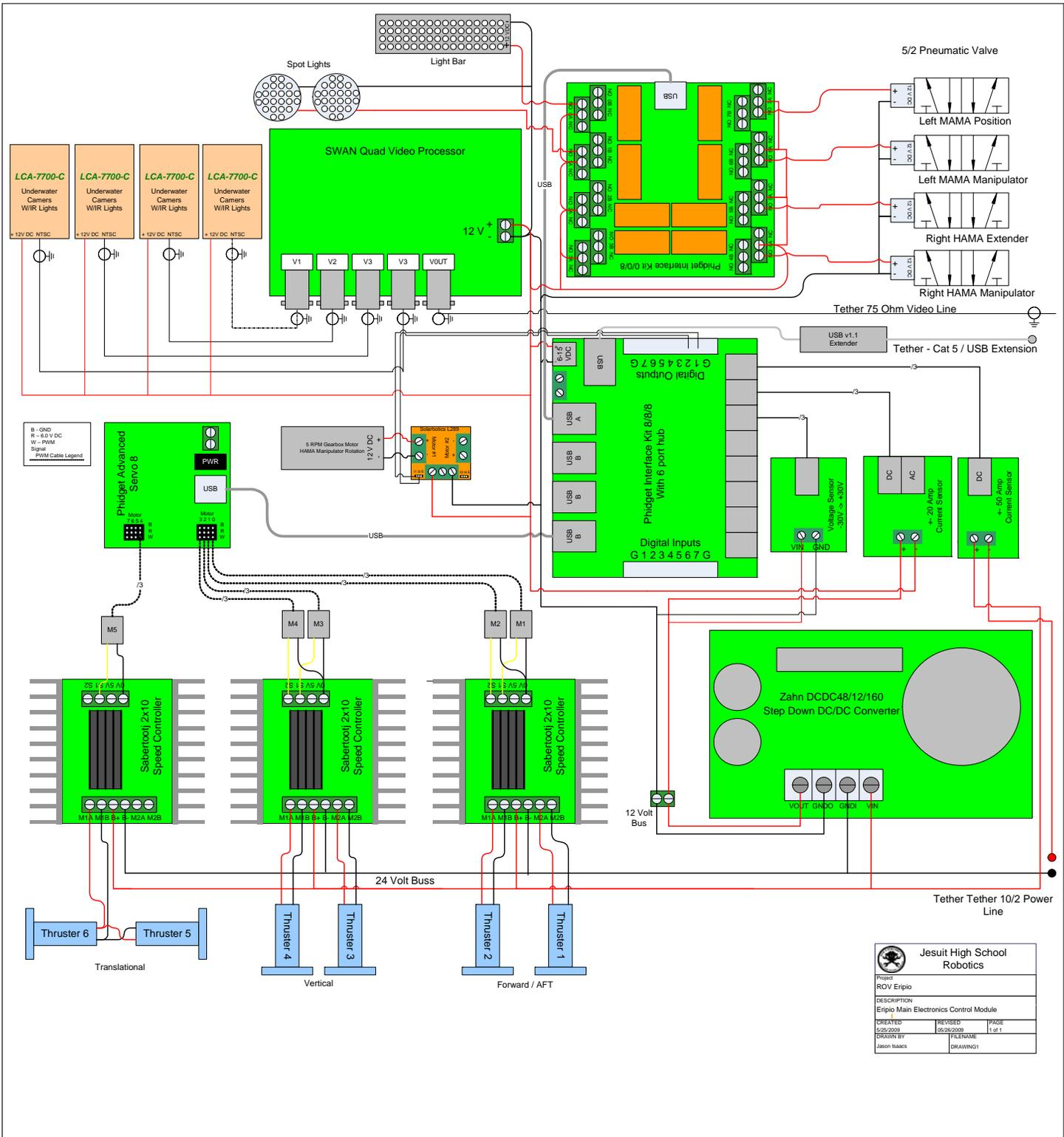
Figure 6 - Eripio's Electronics Control Module Schematic
