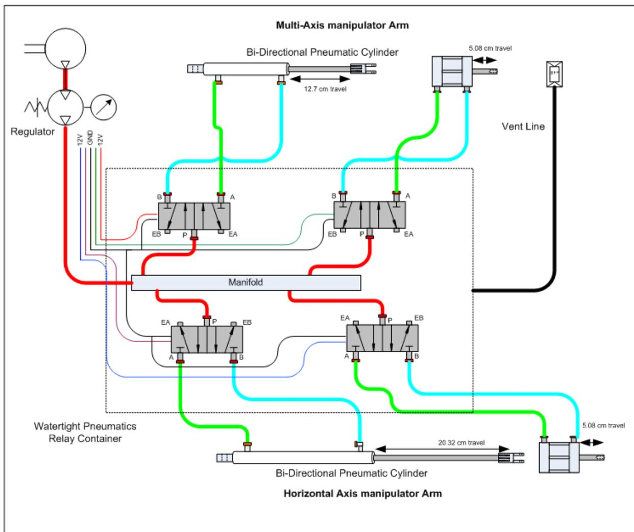
Figure 8 - Pneumatics Control Diagram
