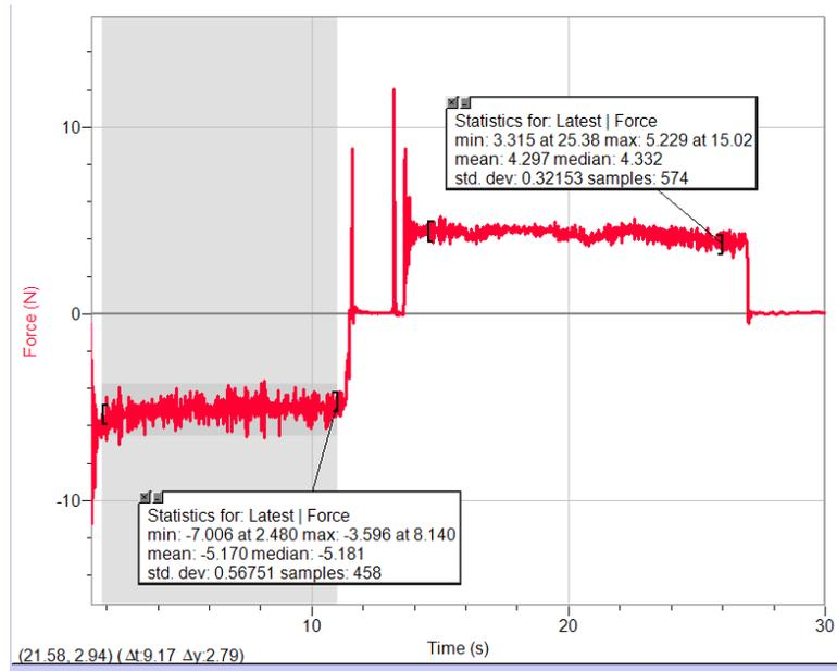
Figure 3 – Translational Thruster Thrust Profile
