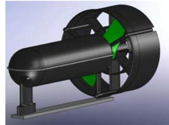
The previous design was to use modified bilge pumps retrofitted with propellers. While this worked well for the prototype, the project needed motors with more torque, as the UROV will be larger and denser than previous designs. 5 SeaBotix UROV thrusters were purchased that are rated for 154.2 meters depth. The layout of motor placement, as well as their resulting motions is as follows:
