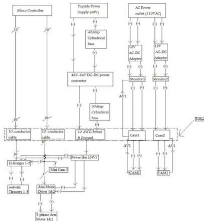
**Fig 7: Schematic Representation of entire power and control systems**
