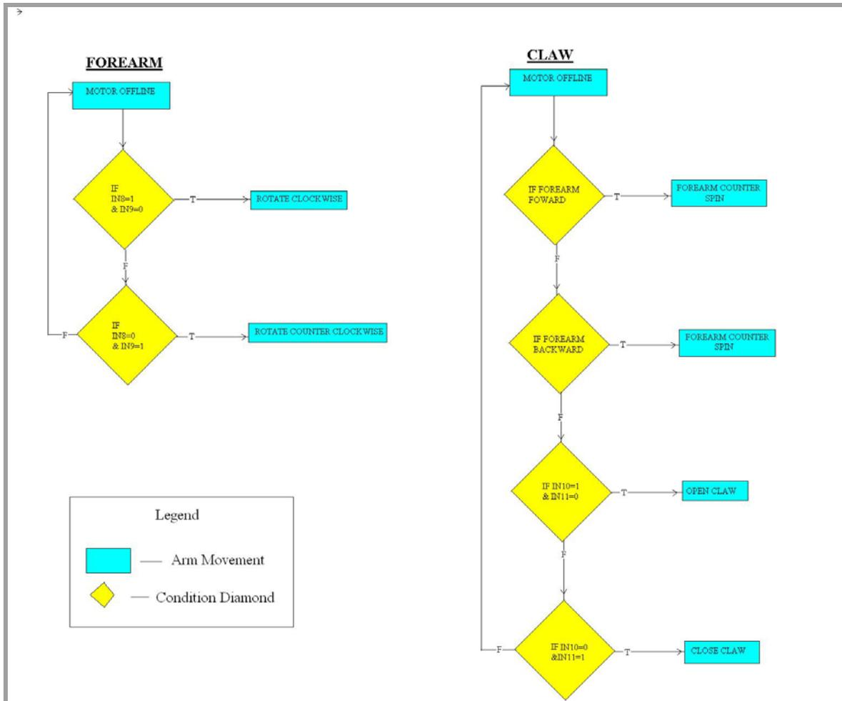
**Fig 12: Software Flow Chart C**
