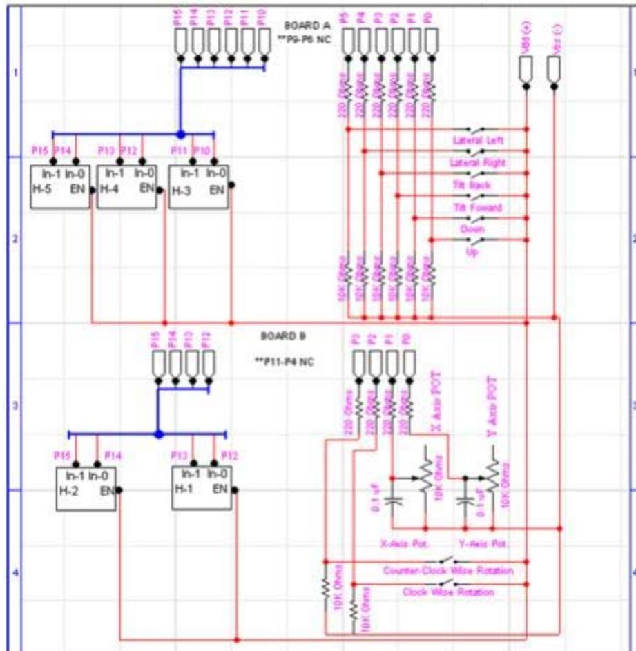
**Fig 8: Schematic for micro-controllers to motor drivers**
