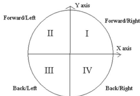
**Fig 9: Joystick (Digital Representation)**
