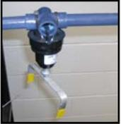
**Tool # 2: Motorized Hatch Opener:** is rear positioned to enable us to unlock and re-lock the hatch. Tool #2 is constructed of a bilge motor, aluminum bar and custom adapter.
