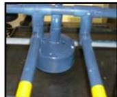
**Tool # 4: Pod Lift Tool:** delivers life-support pods. It is positioned directly below the adjustable ballast system. The Pod Lift Tool consists of two 1/2" PVC pipes.
