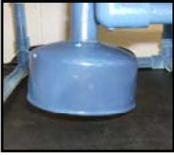
**Tool # 1: Docking Collar:** allows us to dock with the submarine and hold a stable position for 20 seconds. Tool # 1 is fabricated from a 4" PVC cap.
