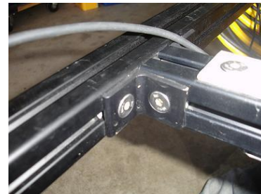
Figure 2 Frame attached together by flathead socket cap screws, ball bearing T-nuts and 90 degree aluminum angle pieces.
