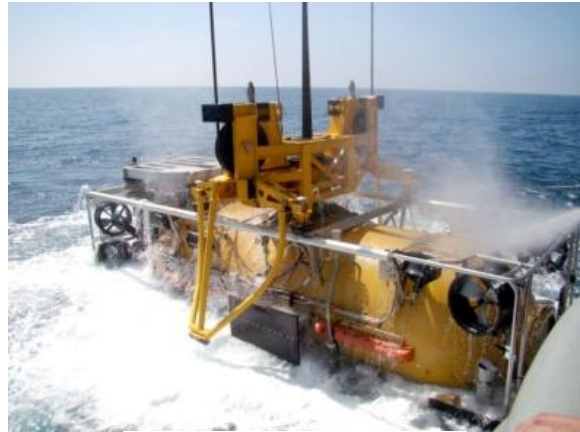
Figure 6 Pressurized Rescue Module
