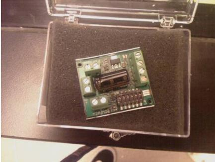
Figure 5. Motor controller used to control the speed of the propellers.
