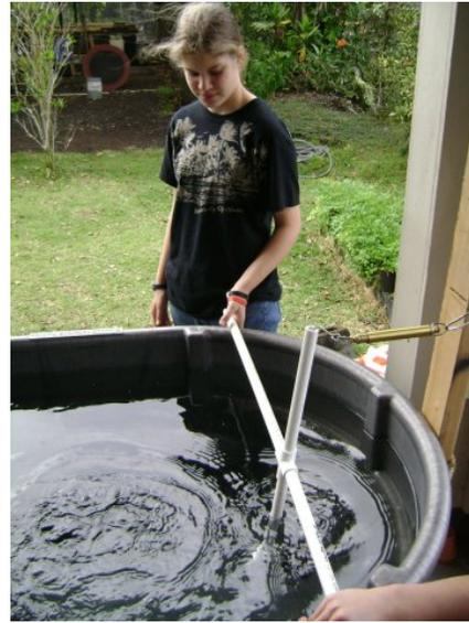
Performing a Bollard test
