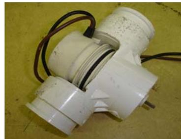
Figure 5: Customized PVC piece for motor
