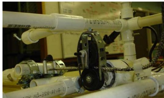
Figure 8: Motorized Pulley System
