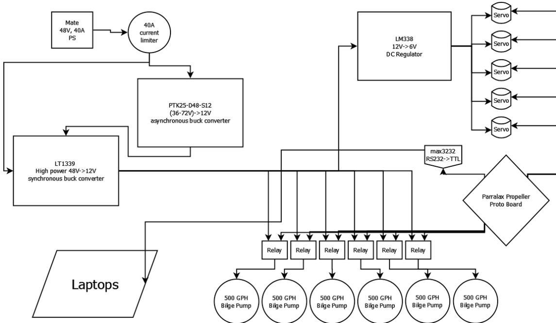
**Figure 3: Electrical Schematic**
