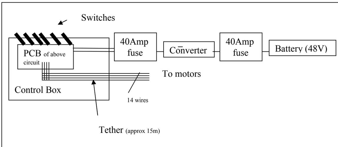
**Figure 7: ROV Controlling System Diagram**
