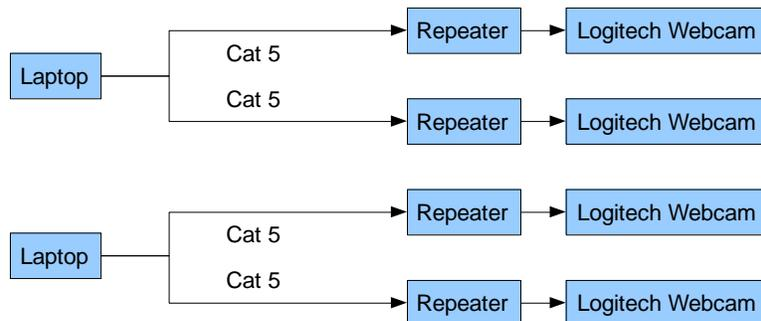
Figure 7 – Camera signal schematic
