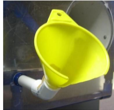
Figure 6 - Ventilation nozzle holster
