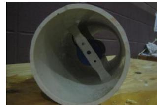
Figure 4 – Tube thruster
