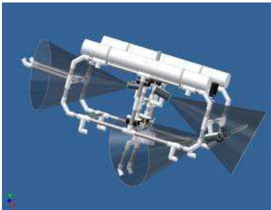
the tusk while also seeing directly in front of the ROV. Our second camera is positioned to view the opposite direction when driving the ROV in reverse. This view also shows the claw. Our last view is aimed at the rotisserie on the bottom of our ROV. This screen is also used to view the skirt when docking with the downed submarine.
