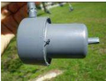
Our ROV uses Rule bilge pump motors. It uses four 4164 liters per hour (1100 gallons per hour) 6 amp bilge pump motors. Our two up and down bilge pump motors are 1893 LPH (500 GPH) and 2.5 amps, while the arm uses a 1363 LPH (360 GPH) bilge pump. All seven of the bilge pump motors are 12 volts.
