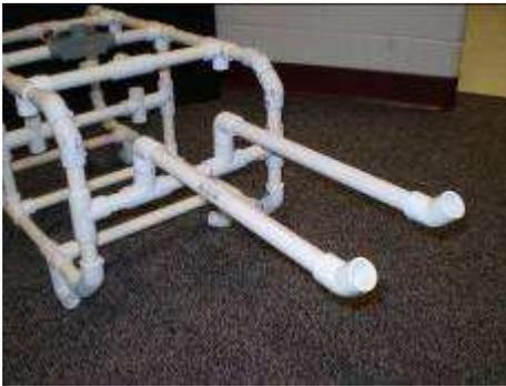
Our tusks are made out of PVC and protrude from the front of our ROV. They are set at the correct height so that our ROV can drive while sitting on the pool floor and maneuver into the Emergency Life Support System (ELSS) pod handles. Therefore, the purpose of the tusks is to transfer the pods from the pod carousel into the open hatch. On the tip of the tusk there is a 45° PVC adapter to prevent the ELSS pods from sliding off of
