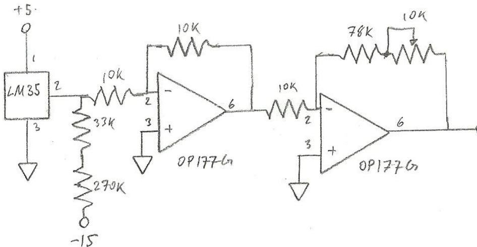
FIGURE 4 - TEMPERATURE READING AND SIGNAL CONDITIONING
