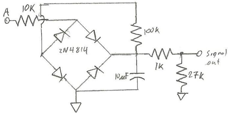
FIGURE 7 - AMPLITUDE CONVERSION
