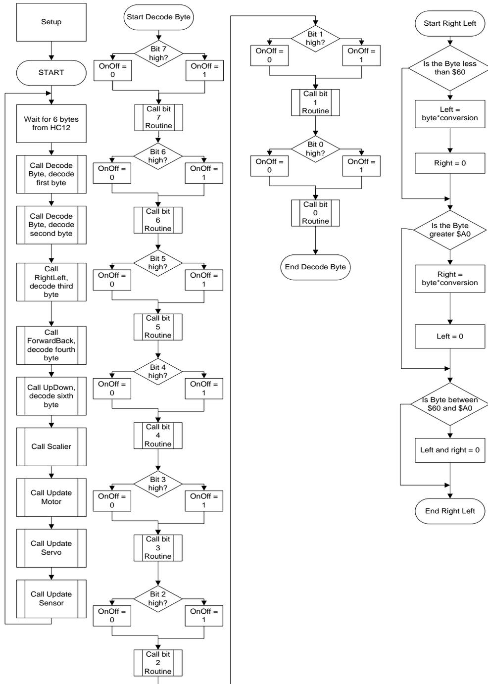
FIGURE 8 - ARDUINO PROGRAM FLOW CHART
