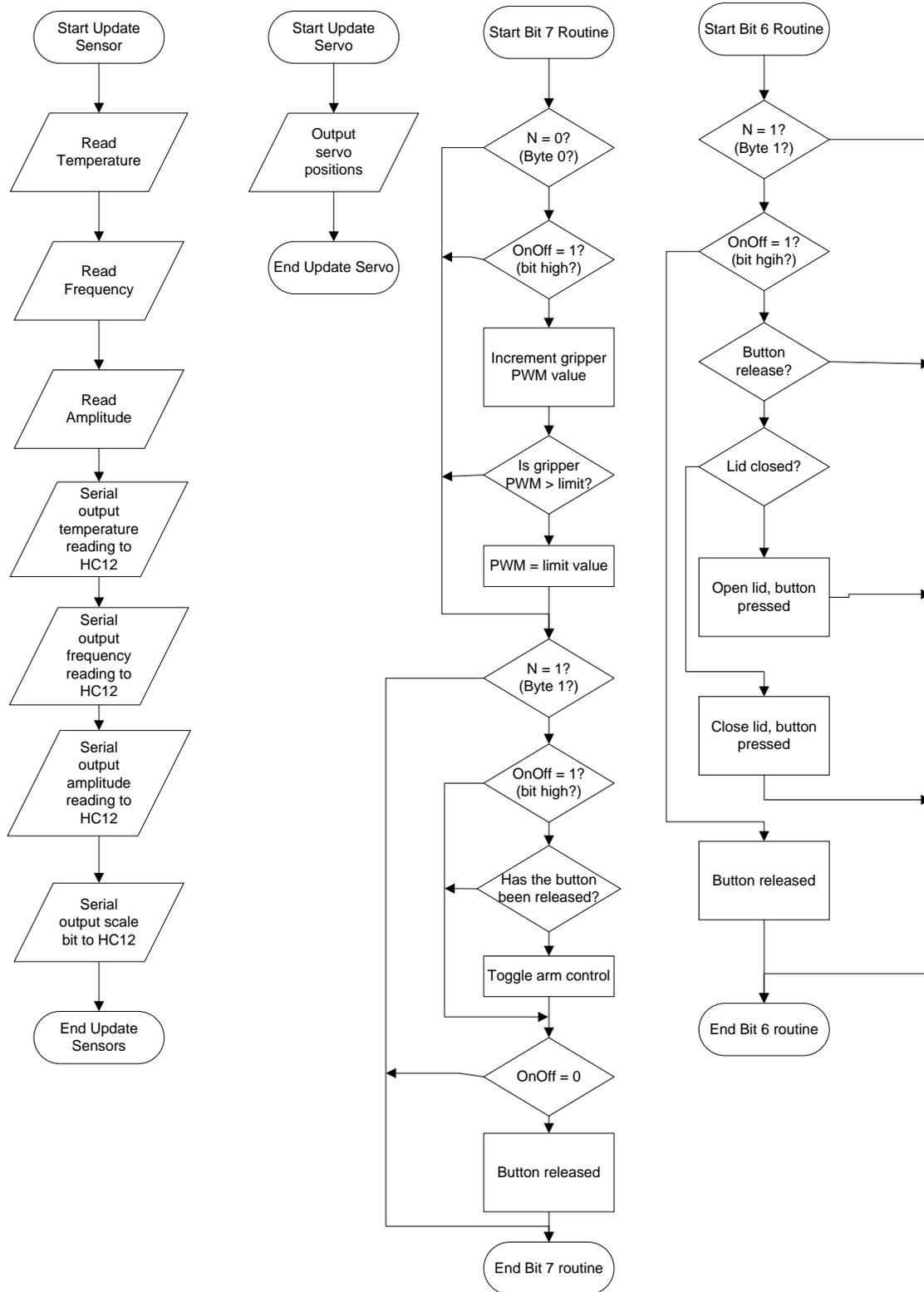
The above flow chart details the processes used by the sensors mounted on the ROV.
