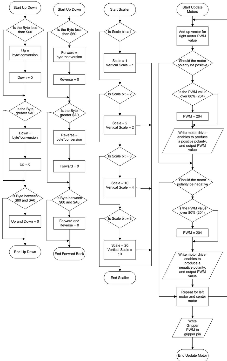
The above flow chart details the processes for controlling the motors.
