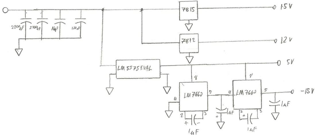
FIGURE 3 - POWER SUPPLY SCHEMATIC
