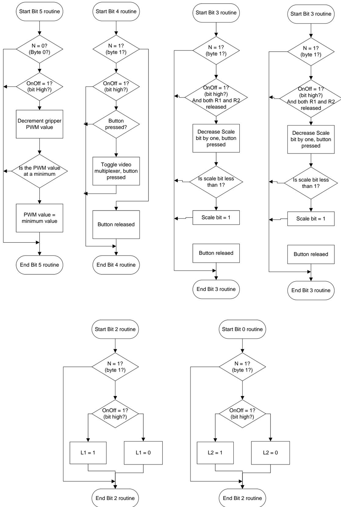
The above flow chart details the process for decoding the control buttons the controller used for the ROV.
