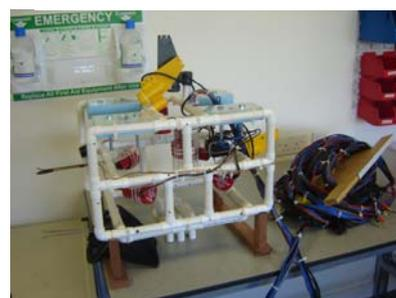
In 2010, the Bucksburn Aquablazers produced an ROV capable of undersea exploration named BUSTER (Biology Undersea Tool for Exploration and Recovery). The design process involved brain storming the mission tasks and sketching out ideas for discussion. A solution was modelled using AutoCAD Inventor which then directed the build of the final ROV. The tooling systems were designed to accomplish the following tasks:
