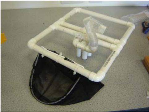
*This shows the dual purpose underside tool for BUSTER. The crustacean net can be seen at the front, with the self vacuum agar tool located in the middle.*
