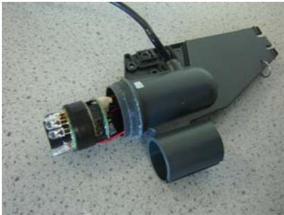
*These pictures show the faulty camera after being disassembled. The PCBs underneath the array of LEDs had a large amount of corrosion and this is probably why the camera ultimately failed.*
