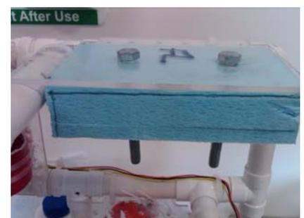
Perspex. Then to achieve maximum stability in the movement of BUSTER these were secured in place in each of the four corners, thus providing an even distribution of floatation. Also these blocks were made to be adjustable by slicing them into evenly thick layers which can be changed depending on the different water temperatures and densities that BUSTER is operating in.
