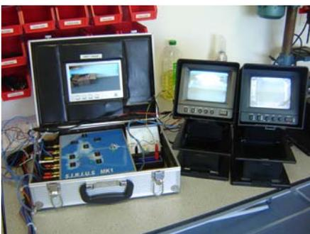
*BUSTER control suite. The colour monitor on the left gives the pilot a frontal view of the terrain whilst the black and white monitors show close up detail of the tooling. The control box houses the two sets of switches for motor control, and also has a voltmeter for temperature readings. The system can provide both analogue and digital readings. Not shown in this picture is the amplifier that allows the pilot to 'hear' underwater. This is located on the right hand side of the colour monitor.*
