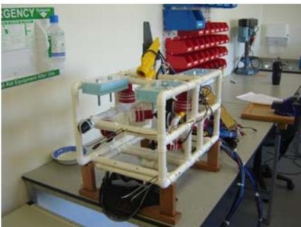
*Front and side views of BUSTER fully equipped with payload tools. Note the wooden stand that prevents damage to the underside tool before and after deployment.*
