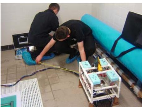
*BUSTER being set up for deployment. Here Ross is setting up the modular control suite whilst Struan is measuring distances along the tether where the flotation collars should be fitted. Through experimentation it was found that these collars should be 1m spaced to make the tether neutrally buoyant. The whole set up procedure can be done in around 3 minutes.*
