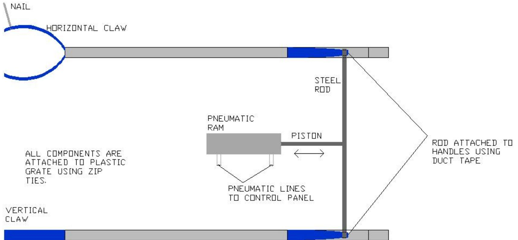
Figure 2: An overhead-view drawing of our pneumatic ram and claw system.
