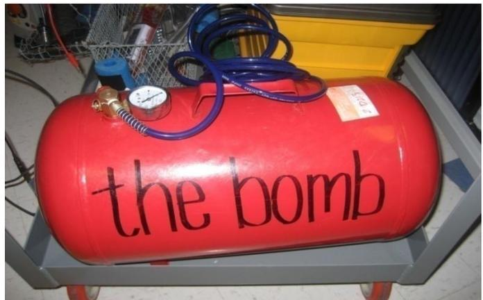
*Figure 6: Air Tank for the operation of our ROV's arms.*
