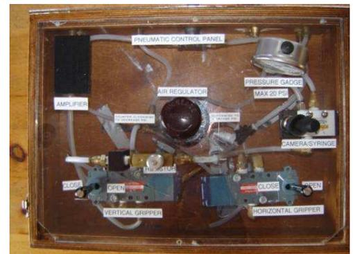
**Figure 13: Pneumatic Control Panel**
