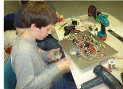
**Figure 6: Constructing the control panel**
