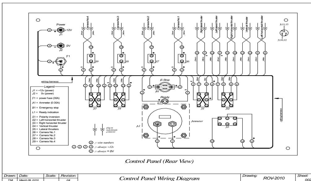
**Figure 9 Control Panel Schematic**
