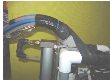
**Figure 5: Tension Relief System**
