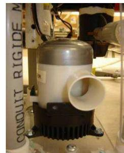
**Figure 12: Lateral thruster in position**
