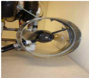
There are left and right motors positioned horizontally and one vertical motor for moving up and down. The horizontal motors are positioned at the back to better manoeuvre and to compensate for the weight of the payload tools at the front. The left and right motors are positioned outside the frame to provide better water flow and to maximize torque for turning. To protect the propeller and personnel, we surrounded the motor with shrouds made from 6" to 7" ductwork
