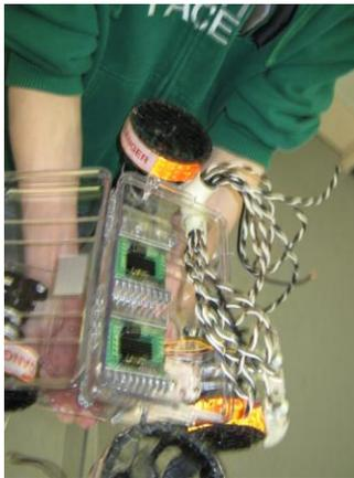
*Figure 7: Watertight box with motor controller*
