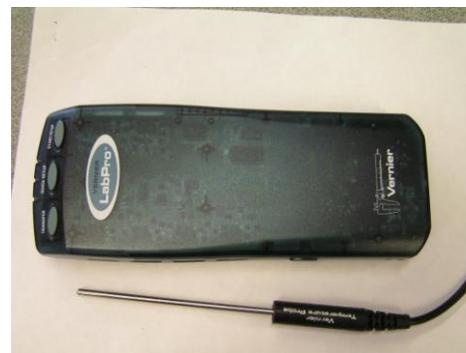
Figure 17: vernier and temperature probe.
