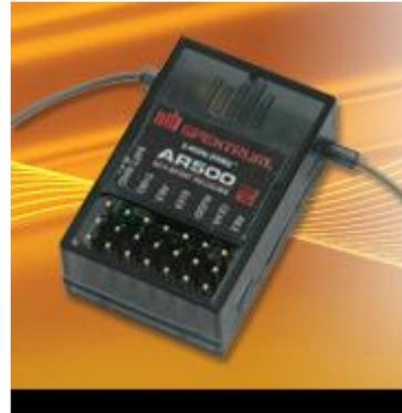
*Figure 5: Remote Control Receiver*
