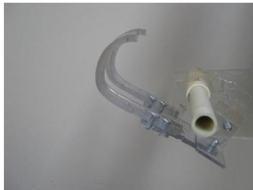
Figure 15: The claw designed out of Lexan.
