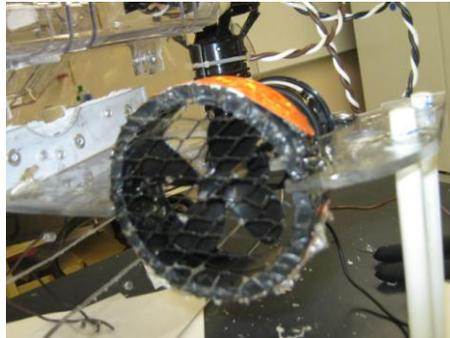
*Figure 12: The epoxyed, mesh on the outside of the thrusters. 4-blade prop shown*
