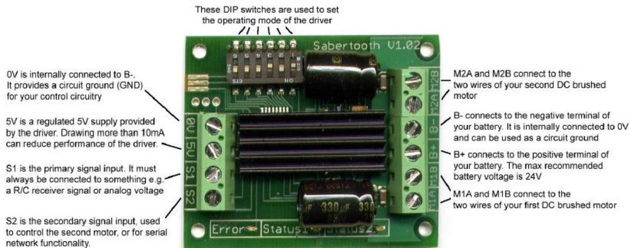
Figure 8: Sabertooth 2x10 motor controllers
