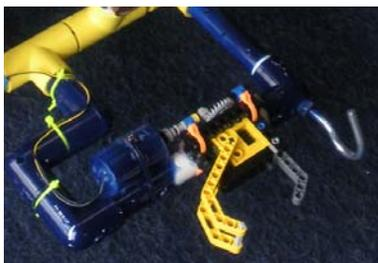
(Photo 8: Hook and gripper tool package)
