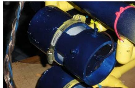
(Photo 3: A motor in its shielding)
