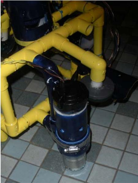
(Photo 11: the Suction Sampler)
