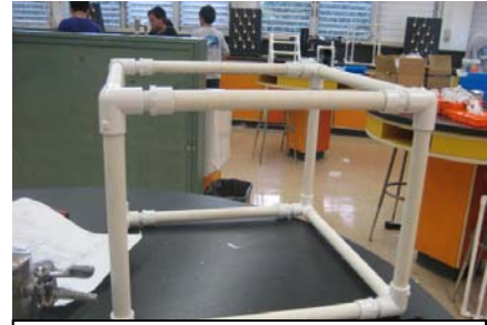
Figure 4: Frame of our ROV
