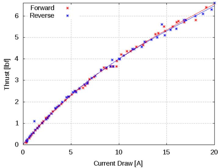
Figure 4 – Thrust to Current Profile of J-3 Thruster
