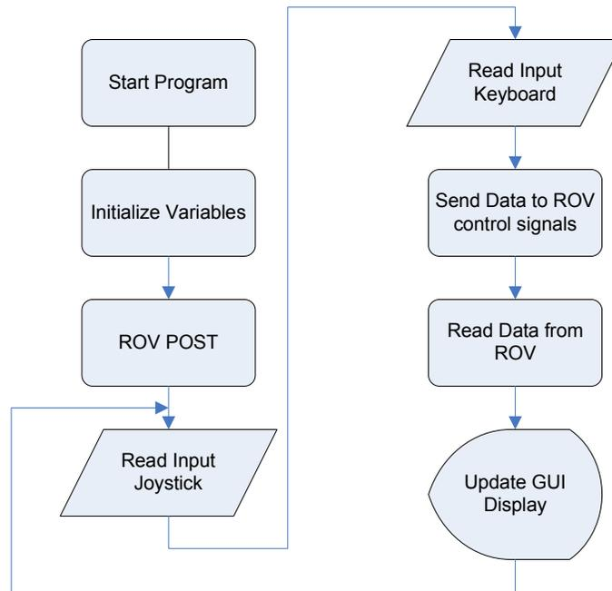
Figure 8 – Software Flow Diagram
