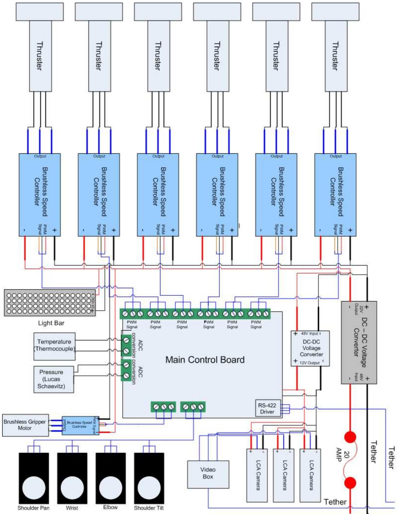
Figure 7 – Electronics Schematic
