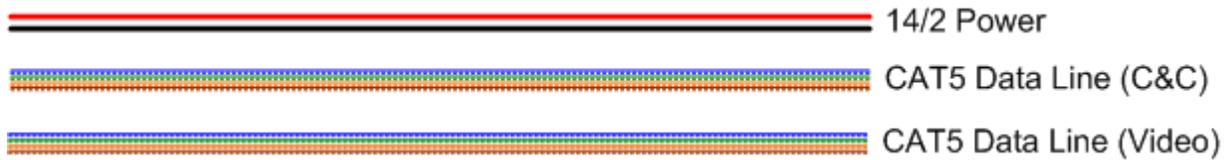
Figure 6 – Tether Diagram
