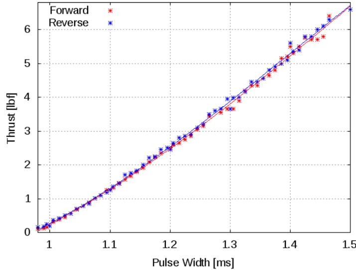
Figure 5 – Thrust vs. PWM Signal of J-3 Thruster
