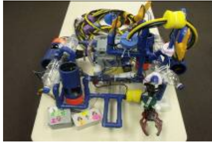
Our ROV with Custom Motor Safety Housings
