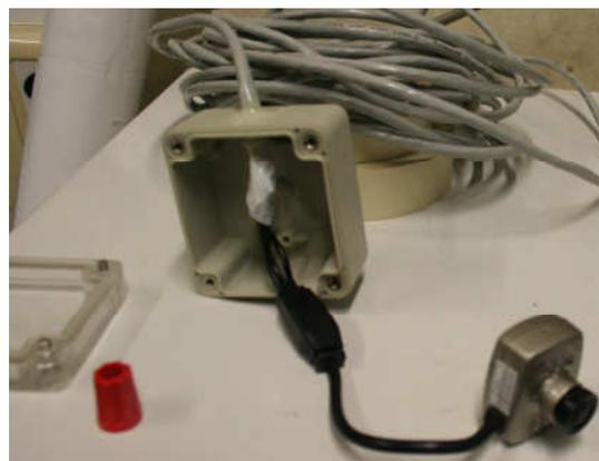
Fig 2.7 – Making of a water-proofed box with Rubber Tubing for Water proof function of the camera
