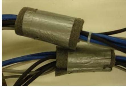
Figure 6: Pipe insulation on tether
