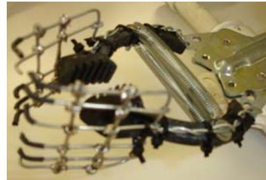
Figure 12: Addition of metal “teeth”
