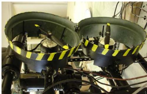
Figure 10: Propeller guards with safety designation
