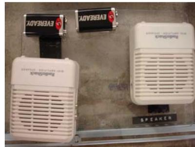
Figure 17: Hydrophone system speakers
