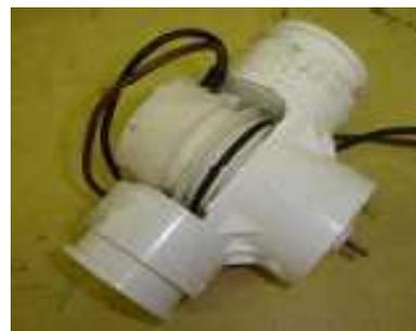
Figure 8: Customized PVC piece for motor
