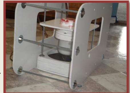
Figure 2 - ROV Rip Tide before payload items and buoyancy installed
