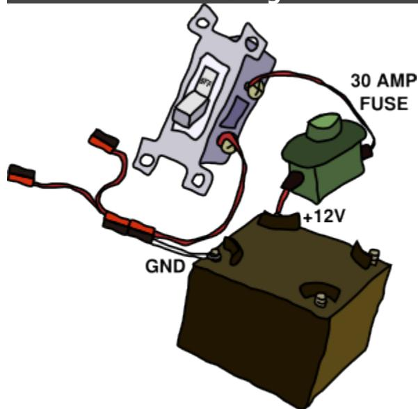
The power system is very simple. 12 volts DC powers both the topside board and the thrusters. Lower voltages are safer and less corrosive for our electrical traces if they get wet while powered up. A 30 amp fuse protects against shorts.
