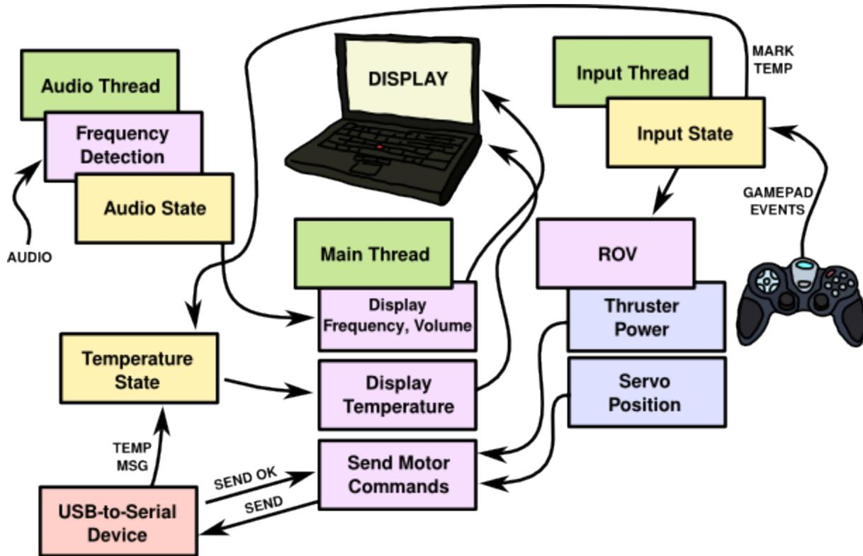
The software on the laptop computer sends motor commands based on user input from the gamepad, calculates the frequency of audio from the hydrophone, and records temperature information from the thermistor. The control software is written in Haskell, a purely functional programming language. Modules from Hackage, a repository of Haskell software packages, are used to handle concurrency, interface with the gamepad, read microphone data, and to calculate the dominant audio frequency.
