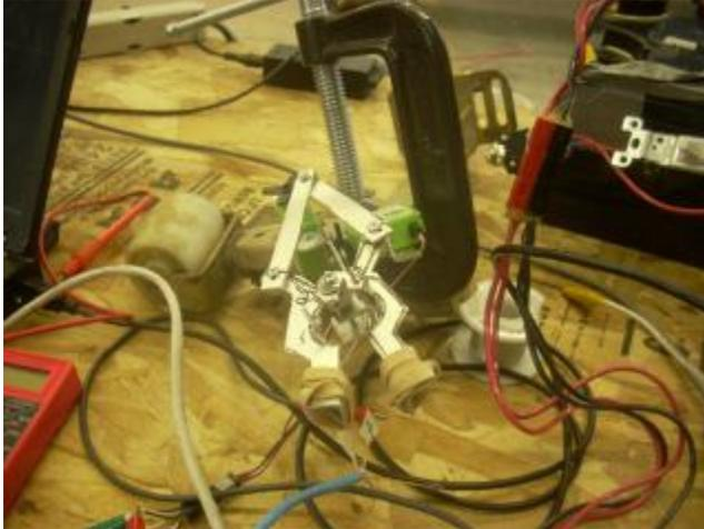
We have two main mission tools at the time of this writing. A piece of cut aluminum in the shape of a fork is mounted to threaded rod on the front of our ROV. With this fork, we can quickly pull the J-bolts from the platform mission. On the other side, we built a manipulable arm out of two servos, sheet aluminum scraps, and some screws. This arm will help us collect the crustaceans in the cave and to carry the "T" from the
