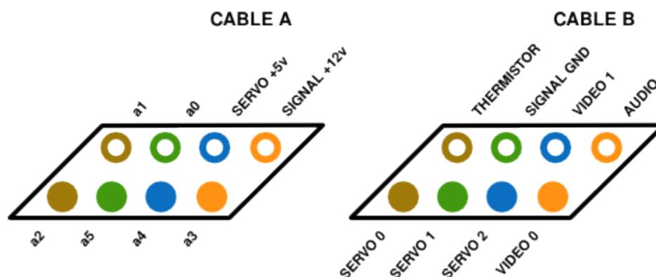
The a[0..5] wires on cable A map to the PIC's PORTA register. The PIC can't supply enough current to drive the relays on the ROV itself, so it signals a row of transistors through a row of 1K $\Omega$  resistors in order to step up the current on the motor control wires. The 6 motor control signals run alongside servo power and motor control ground on cable A.
