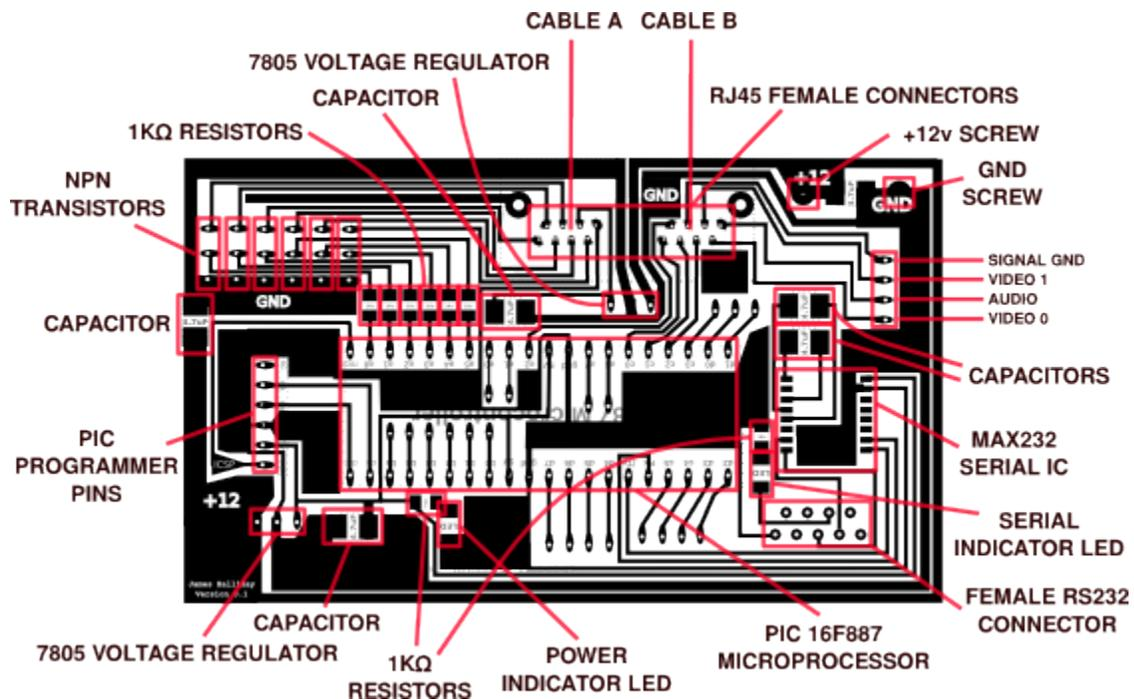
The topside circuit board sits near the laptop computer above the water and communicates with the computer through a serial-to-USB cable. Signals from the serial cable are managed by the MAX 232 serial chip, which is wired into the TX and RX pins of the PIC 16F887 microprocessor. The topside board has two female RJ45 connectors for the cat5 cables coming off the tether.
