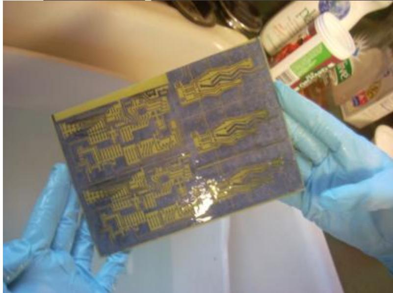
Using this method, we were able to etch multiple relay and topside boards onto a single sheet of copper-clad fiberglass in an afternoon. Both the relay and topside board schematics in the previous sections minus the red labels are the actual images we used for etching.
