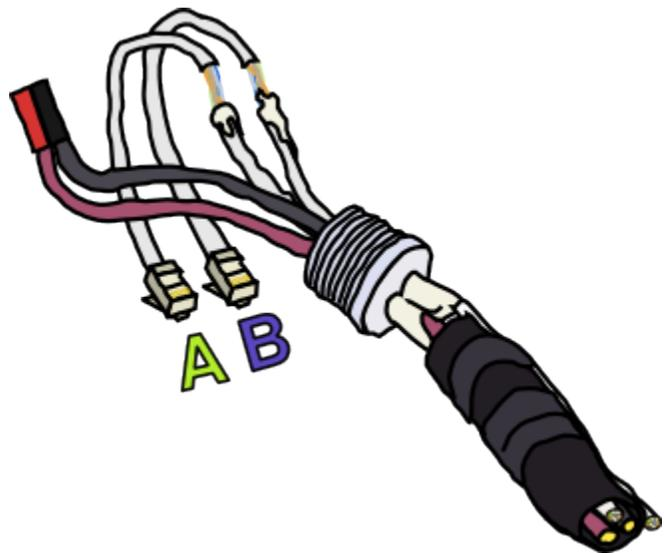
The end of the tether has PVC screw thread that hooks into the electronics housing, where the cables are routed internally.
