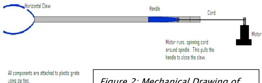
*Figure 2: Mechanical Drawing of Manipulator Subsystem*
