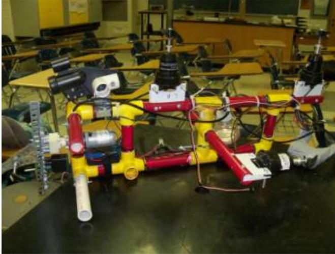
Figure 6: Structure of the ROV in process. As you can see, it does not have a full frame but rather a backbone, supports, and wings.
