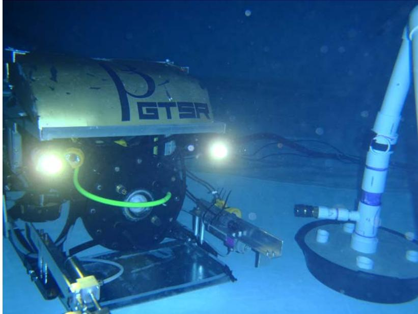
Georgia Robotics Technologies introduces ROV Beta as a new mobile oil spill emergency response platform. Leading the response to the Deepwater Horizon Oil Spill, ROV Beta leverages new technologies to remove damaged riser pipes, cap oil wells, collect samples, and perform other underwater scientific and engineering tasks.
