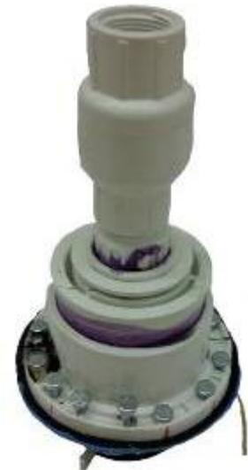
*Figure 17: Wellhead Cap Prototype 4*
