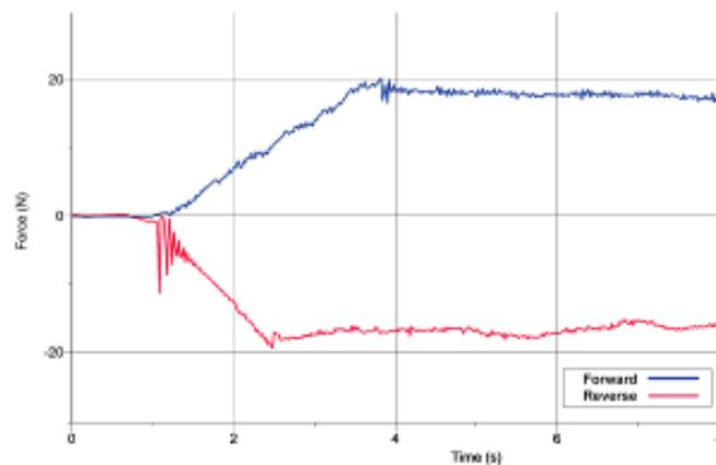
Figure 3: Seabotix™ Thrust Profile
