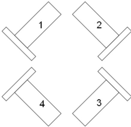
Figure B-1: Thruster Configuration on ROV
