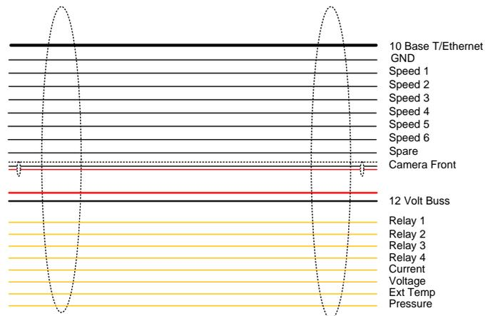
Figure 6: Wire diagram in conduit
