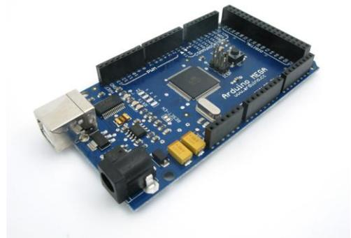
*Figure 9: Arduino Mega*
