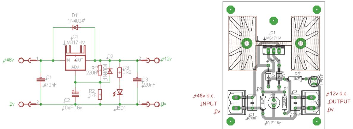
Figure: Voltage Regulator (48Vdc to 12Vdc)
