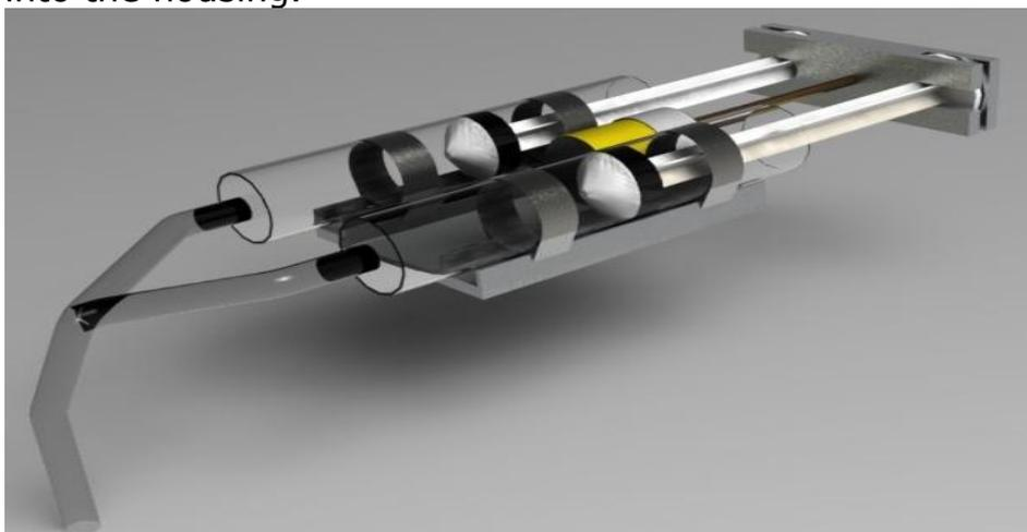
**Figure: Final water sampling tool**
