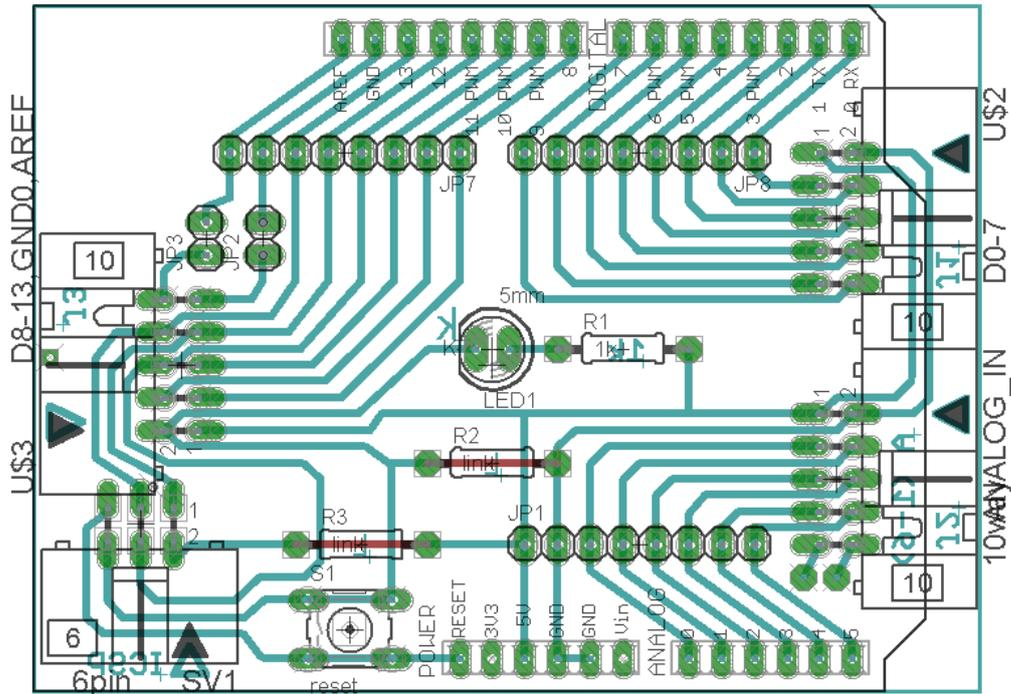
Arduino Duemilanove 10 way connectors shield board layout (prototype 1)
