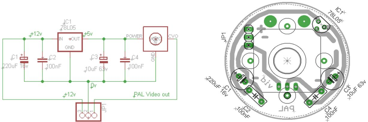
Figure: Camera circuit
