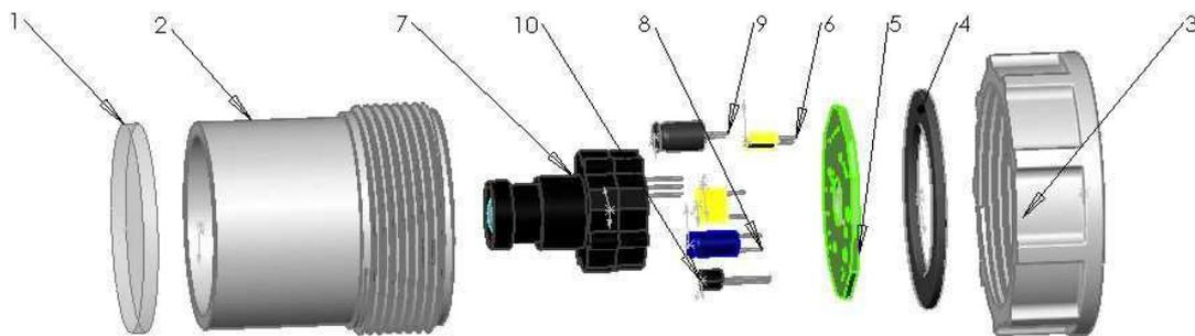
Figure: Camera external housing
