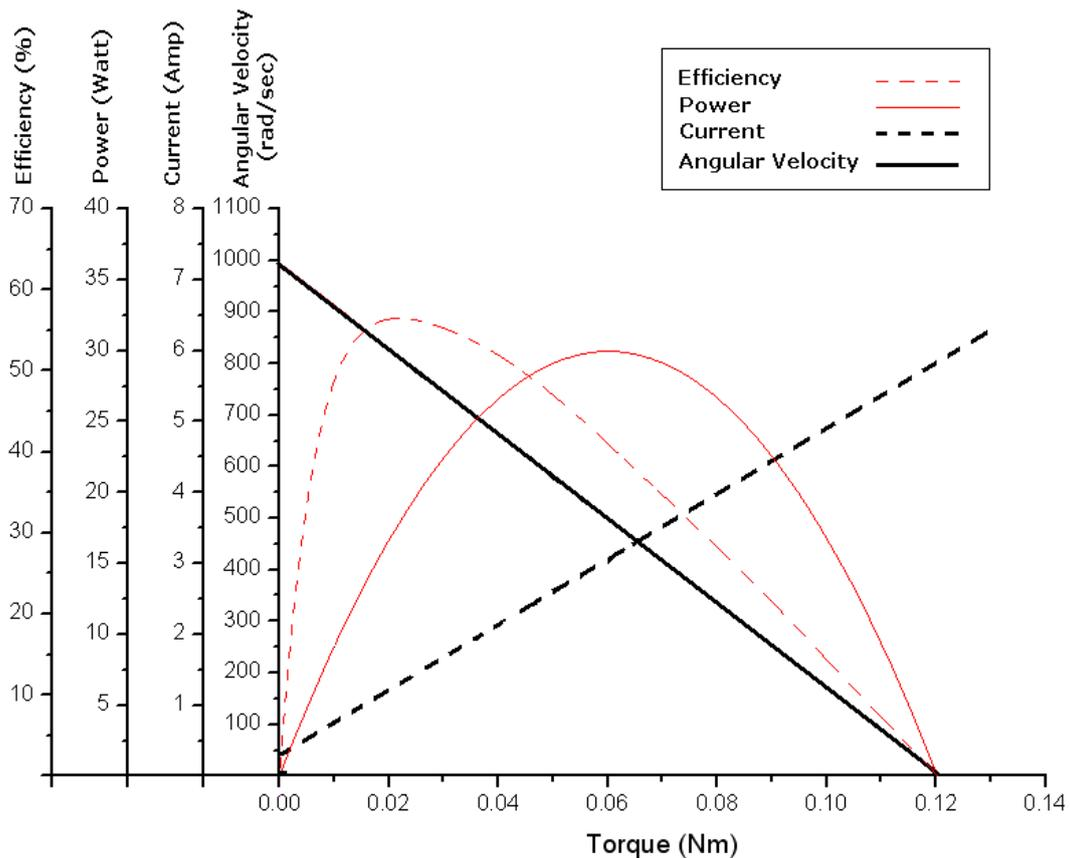
**Figure: Submersible motor performance curves**
