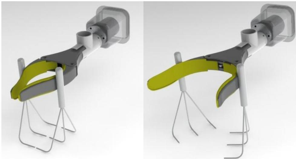
**Figure: Open and close configuration of the grabber with claws attached to it**
