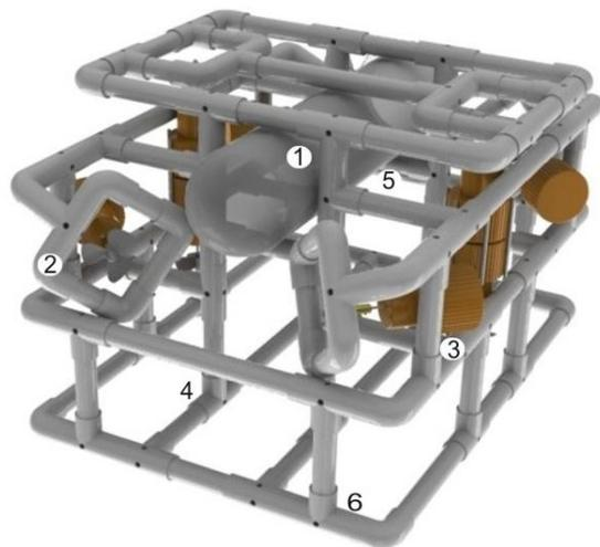
The frame was designed and build by the company members using hand tools. Due to the symetrical construction of the vehicle, the frame was divided on modules and each of them was built separately. Once all were built, the frame was assembled together. Then, holes were drilled on the frame to flood the frame once it is in water. Also all the joints were secured with tap screws.
