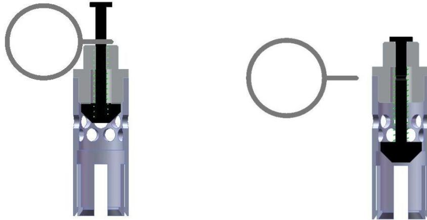
**Figure: Cross-section view of the open and close configuration of the cap**
