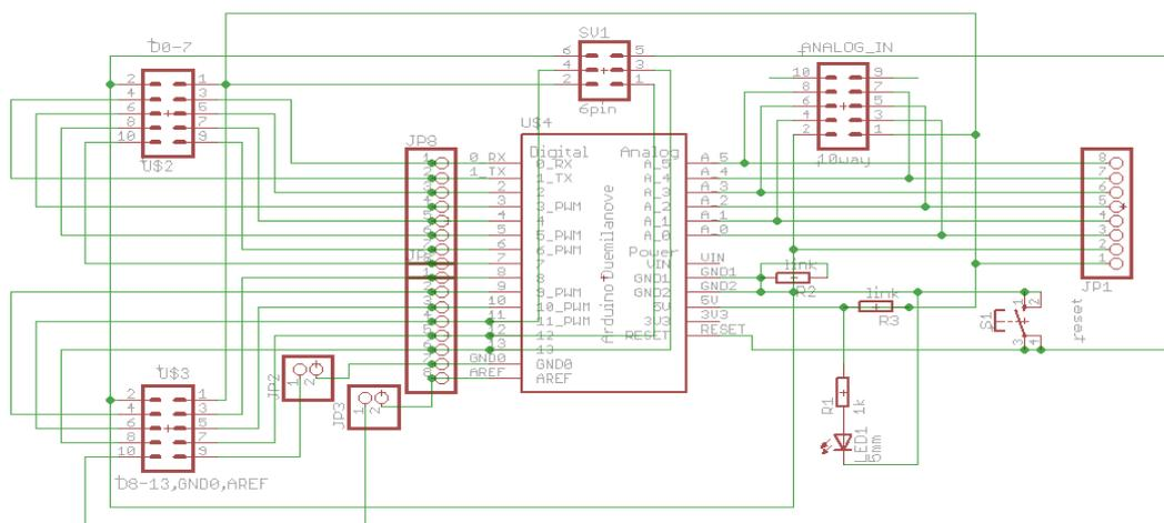
Figure: Duemilanove 10 way connectors shield schematic diagram (prototype 1)
