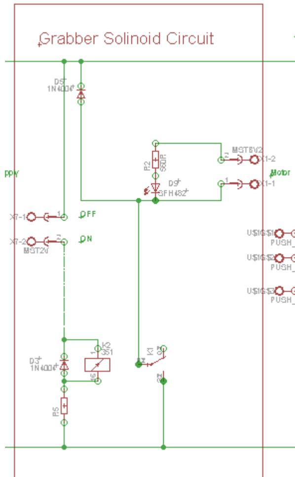
Figure 2 is the control circuit for the grabber. The circuit consists of a simple relay switching configuration. When the switch is set at the off
