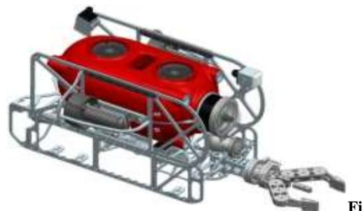
Figure 1 - A CAD model of the Omega ROV
