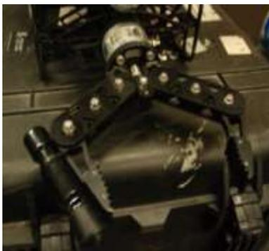
Figure 3: Manipulator attached to The ROV
