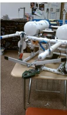
**The Harpoon** - Drilling a hole through a PVC cap and sliding a threaded rod through constructed harpoon. The rod was held in place by the use of two washers and lock nuts tightened to each side of the cap. The cap was placed
