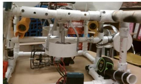
**Camera 2-** This camera is mounted on the left side of the ROV viewing the metal detector, compass, and the manipulator. This camera is used when we are close to a task and using the tools.
