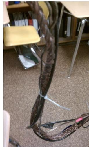
bilge pumps, three camera wires, and one wire for the lateral thruster, and one for the manipulator.
