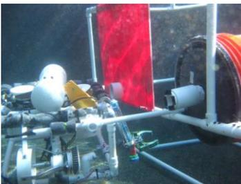
**Manipulator-** The Manipulator was designed to remove the coral from the work surface of the ship and replant it in the grid next to the ship. We used a VEX manipulator, powered by a VEX motor. The motor is wired to a 5-speed controller so that it can be opened and closed at a speed that is controllable. The Manipulator is also important so that we can retrieve dropped items from the pool floor.
