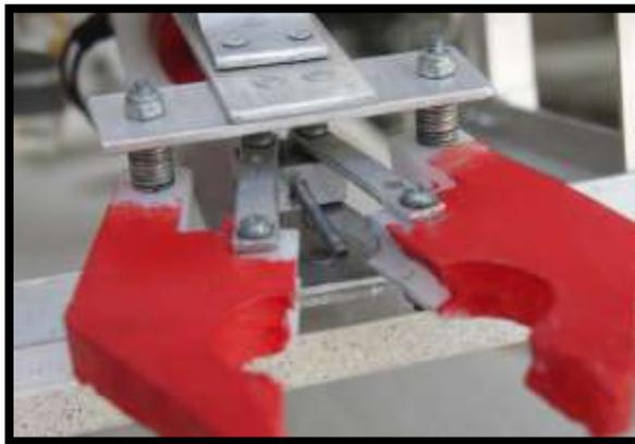
**The linkage used to convert rotational to linear movement can be seen in the middle of this picture, between the two jaws**
