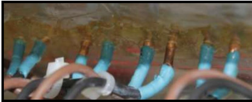
Through-hull connectors inside the Otterbox®. These connectors lead to the thrusters.
