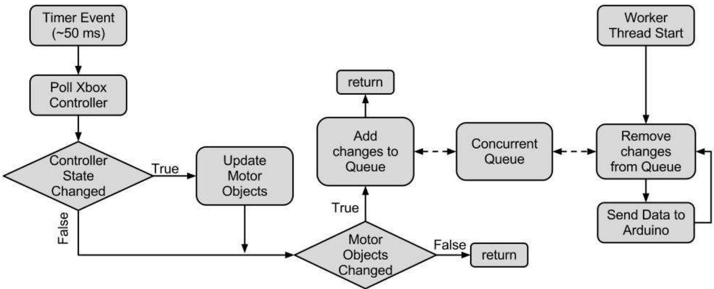
Flowchart for program running on the Arduino
