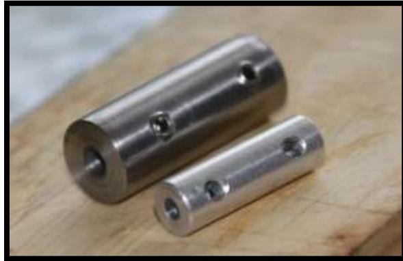
**The new custom machined steel coupler (back) and the old commercial aluminum one (foreground)**
