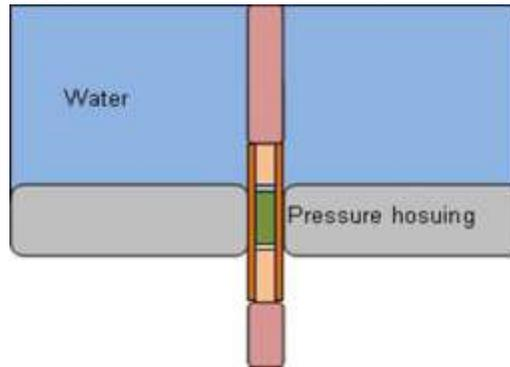
**An illustration of the through hull connectors devised by the company. The green is the epoxy plug, the light brown is the wire, the dark brown is the copper tube, and the light red is the insulation on the wire.**
