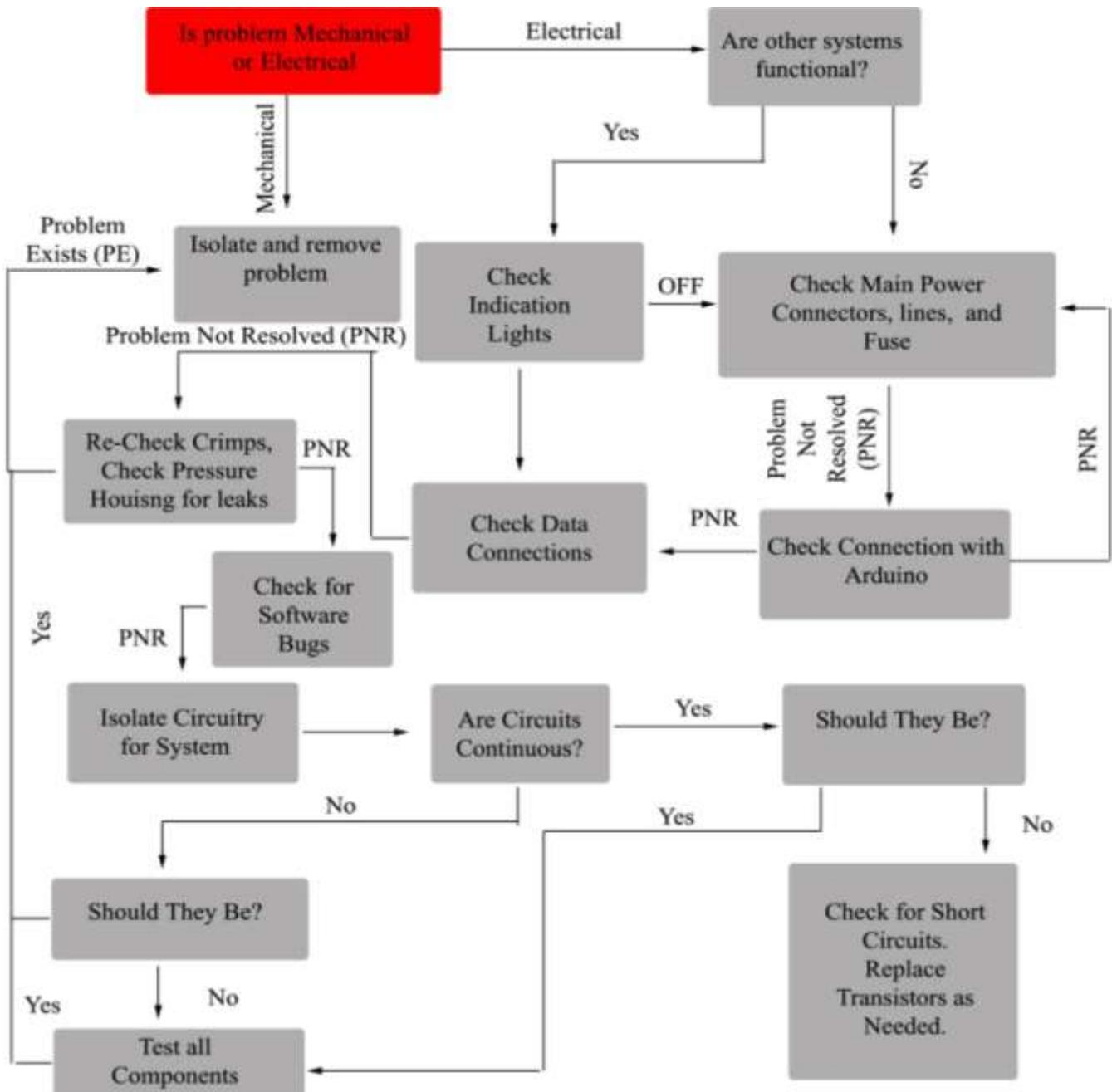
flowchart is used to diagnose and fix mechanical and electrical problems on our ROV, and has been successful for identifying a variety of problems over the development season.
