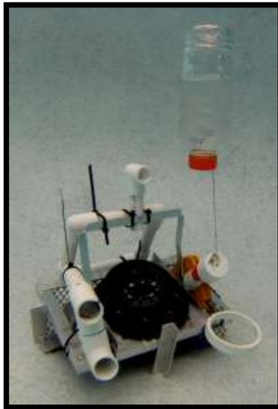
From left to right: the ultrasonic thickness gauge and neutron backscatter device, the compass and the tape measure in the ROV's tool basket.
