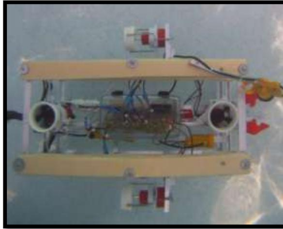
The final pressure housing is located in the middle of the robot and is visible in this picture.
