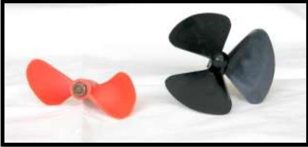
The old 2-bladed propeller (left) and the new, 3-bladed Kort propeller (right)
