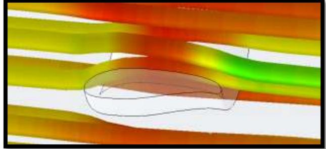
This picture shows a computational fluid dynamics analysis of our nozzle profile in Solidworks©. The tubes reflect the path of water around the nozzle, and the colors indicate the relative speed of the fluid at different points in its flow through the nozzle.
