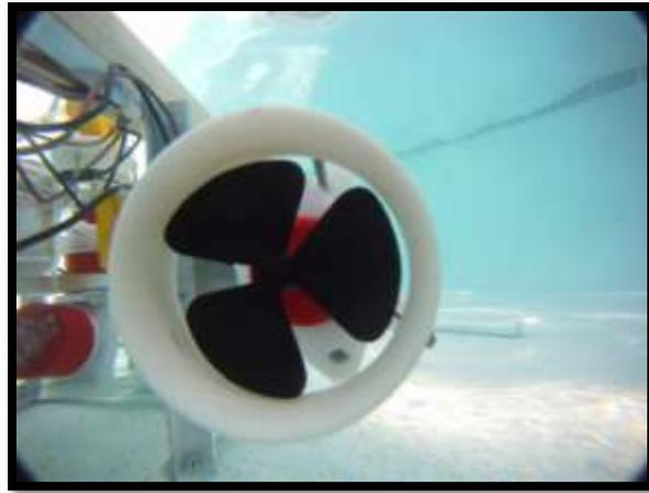
The nozzles mounted with the Kort props attached. In the final nozzle configuration, less than 1 mm of clearance exists between the ends of the propellers and the interior of the nozzle.
