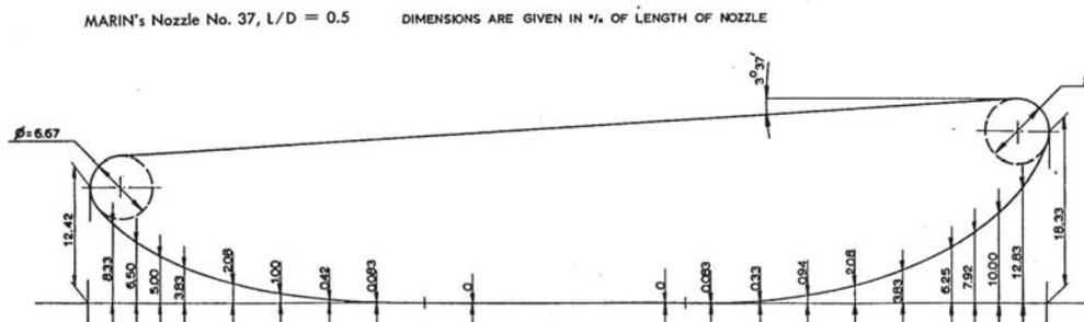
Figure 4: Profile of Kort nozzle used in thruster
