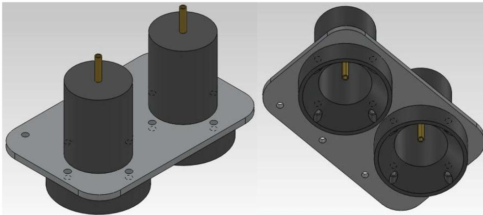
**Figure 8: Top view (left) and bottom view (right) of fuel extraction device showing brass tubing used to penetrate petroleum layers. The cones are shown in the bottom view and are inside the hollow cylinders**
