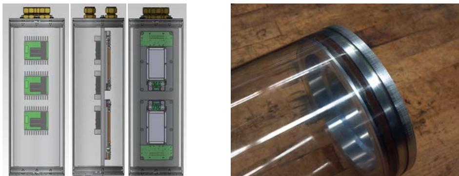
**Figure 2: SolidWorks model of the motor control capsule which includes three motor controllers and two Vicor power converters (left). An end cap for the electronics capsule is shown with O-Ring and polycarbonate cylinder (right).**
