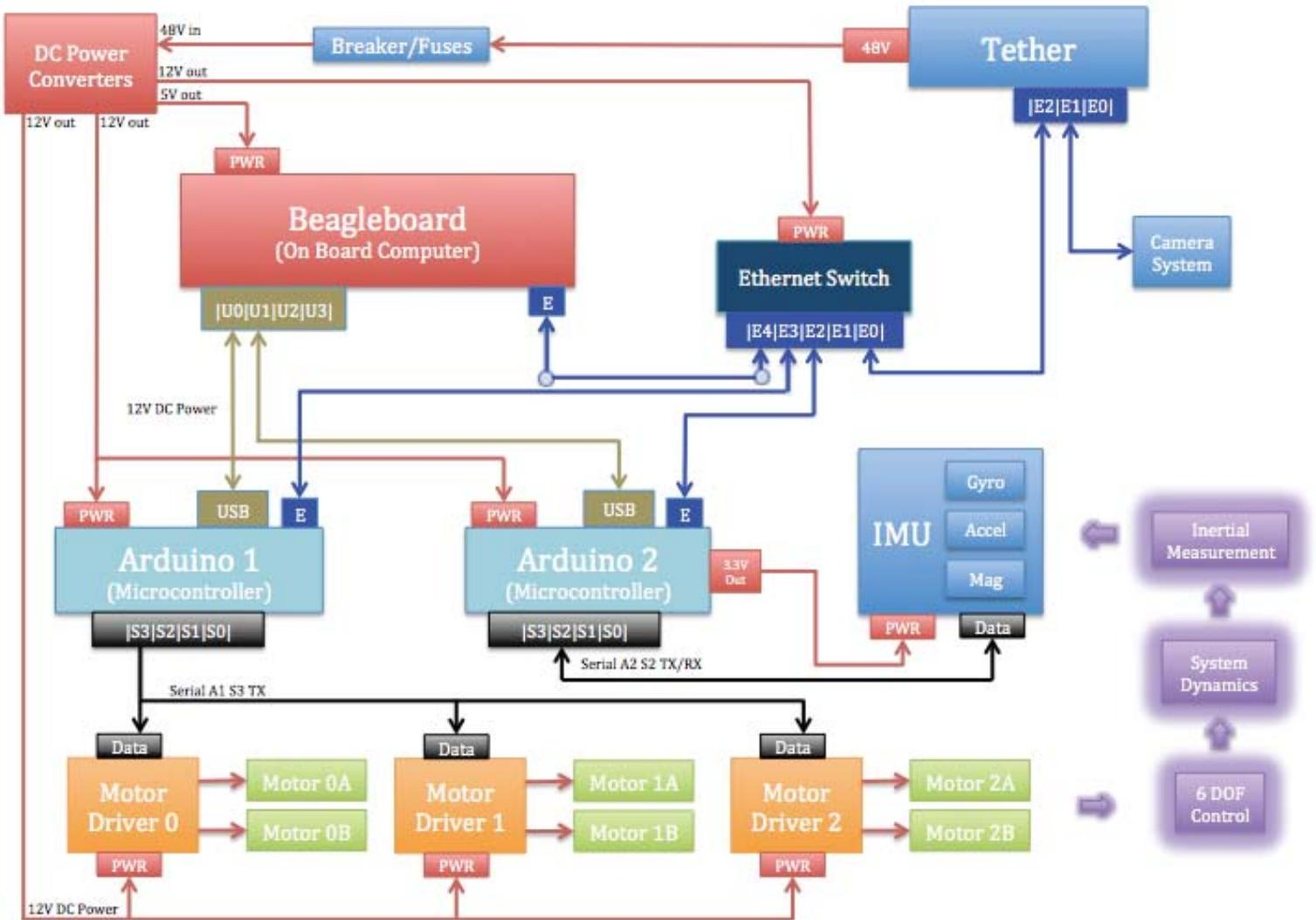
Figure 11 Electrical schematic showing connections between electronics.
