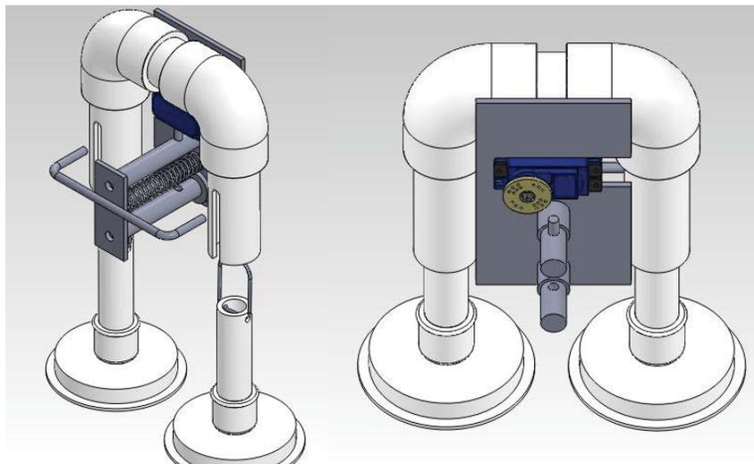
**Figure 9: Front (left) and back (right) views of capping system, showing servo and pin system as well as spring to release sealing caps**
