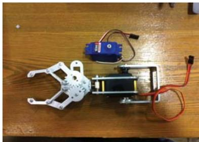
**Figure 7: Manipulator arm with servomotor**
