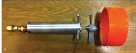
Figure 3: UNH ROV Thruster partially assembled
