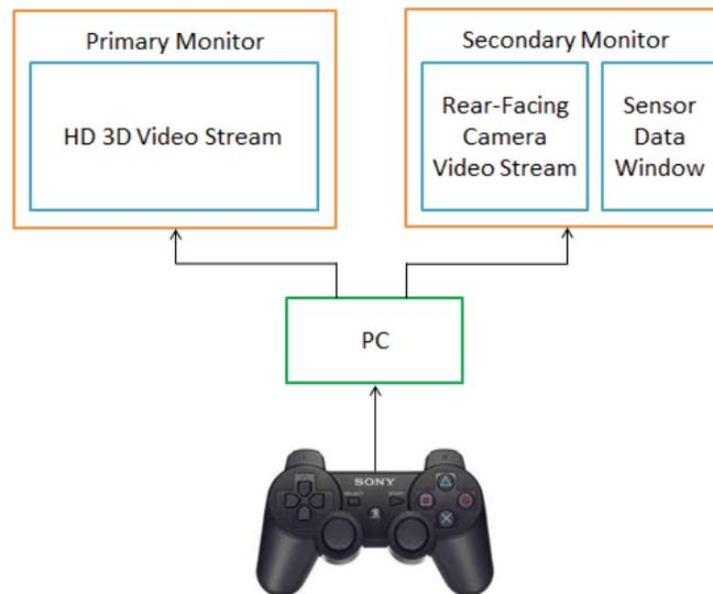
**Figure 13** Digital user interface utilizing a PS3 controller and 3-D vision.
