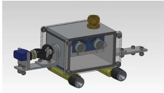
**Figure 6: Front view of SolidWorks model of camera housing. Servo motor and damping coupling is shown on the left and two flashlights are connected to the bottom of the camera box. The two cameras facing forward are shown also.**
