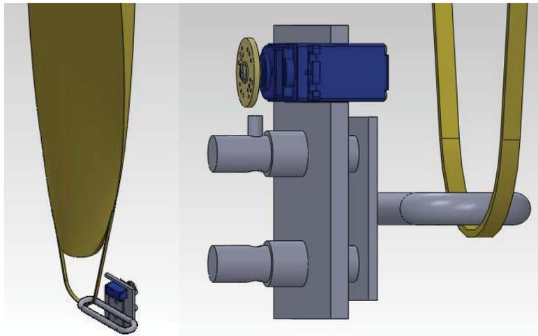
Figure 10: Lift bag system (left) and connection to ROV (right)
