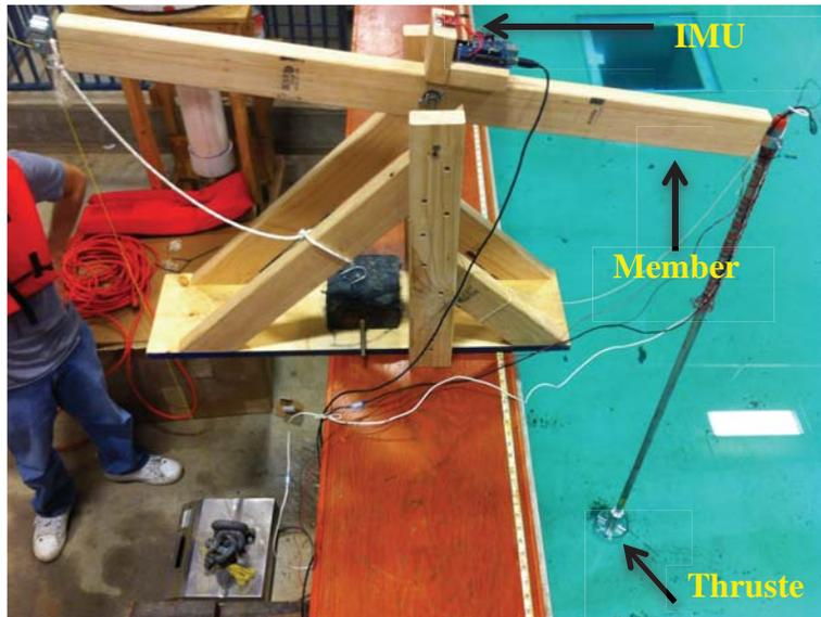
**Figure 14** Teeter totter assembly to measure thrust and debug/develop PID control system. The IMU was located in the center of rotation.
