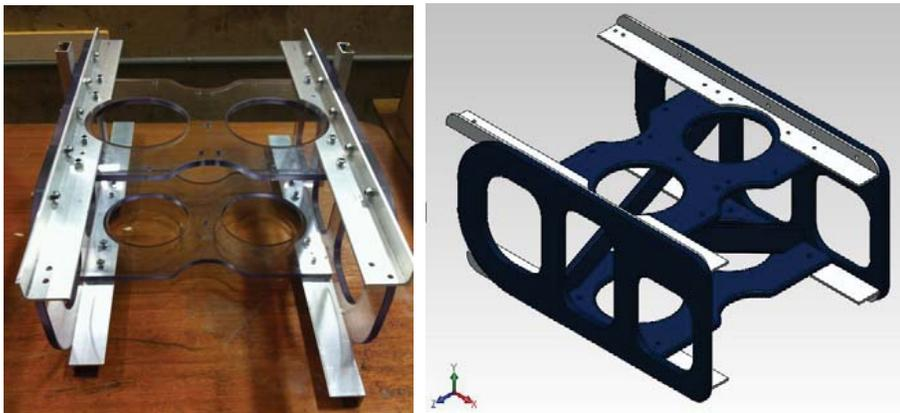
Figure 1: Fabricated chassis frame and SolidWorks frame model
