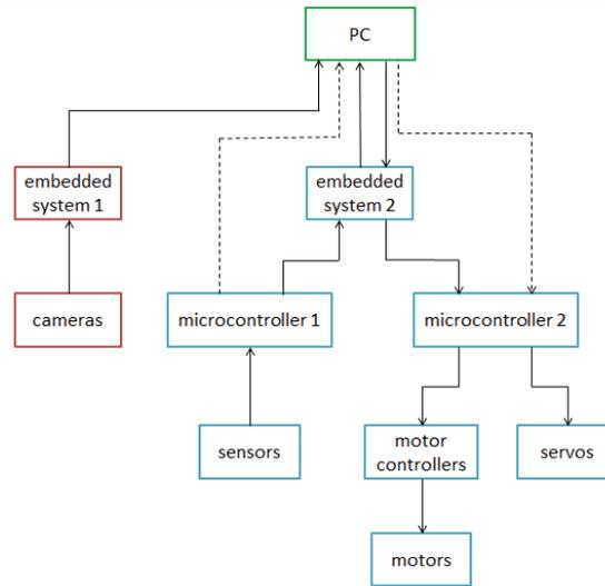
**Figure 12 Software flowchart where solid arrows indicate primary data paths, while dashed arrows represent backup connections.**
