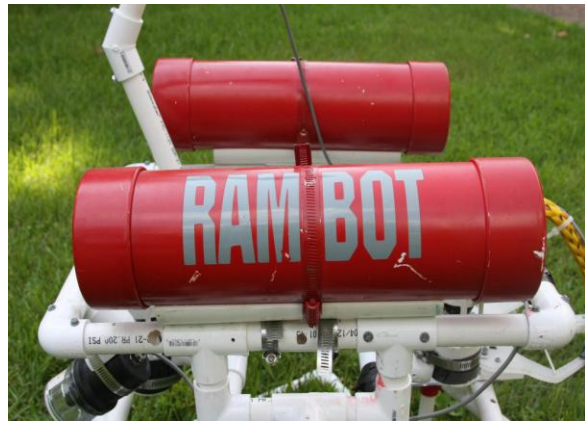
Top: Rambot’s ballast for buoyancy made from 3” sealed PVC pipe Bottom: Lead weights on frame to add mass
