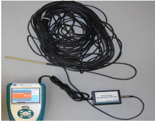
Extra long temperature probe with Vernier LabQuest
