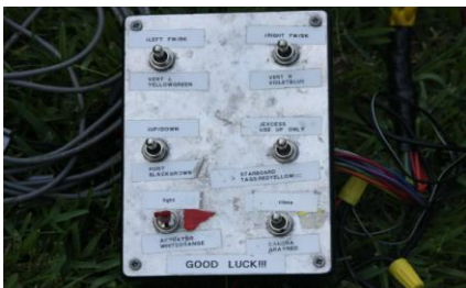
Rambot control box with double pole – double throw switches
