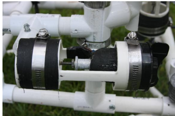
Top: Bilge motor with propeller Bottom: bilge motor with protective housing
