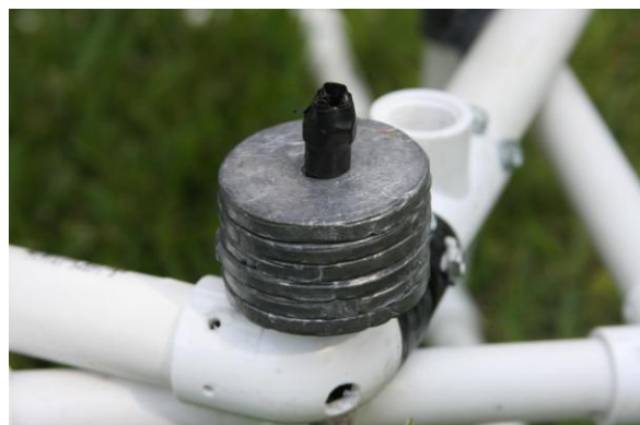
Top: Rambot’s ballast for buoyancy made from 3” sealed PVC pipe Bottom: Lead weights on frame to add mass
