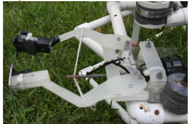
Rambot Gripper powered by a bilge motor allowing for open and closed positions
