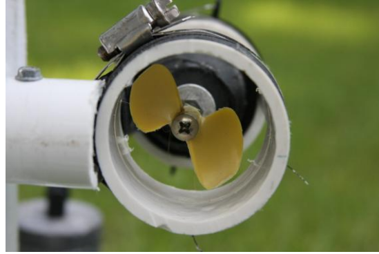
Top: Bilge motor with propeller Bottom: bilge motor with protective housing
