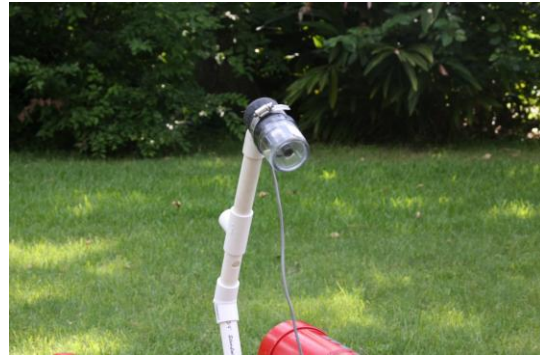
Top: Rambot camera mounted above ROV gives view of where ROV is headed Bottom: camera positioned to view arm
