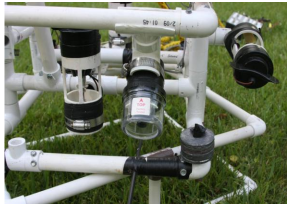
Top: Rambot camera mounted above ROV gives view of where ROV is headed Bottom: camera positioned to view arm
