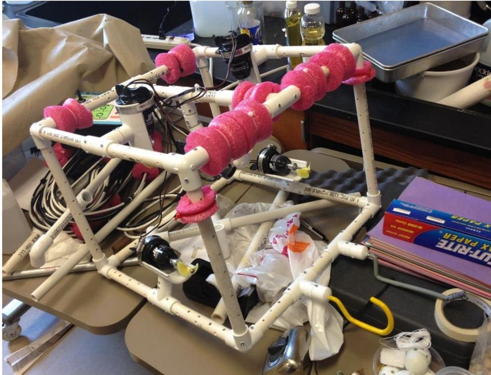
The Aquatic Eagle ROV, pictured above, features a sturdy and lightweight pvc frame reinforced with screws, four motors, an underwater fishing camera, two hooks, and pool flotation tubing for buoyancy.
