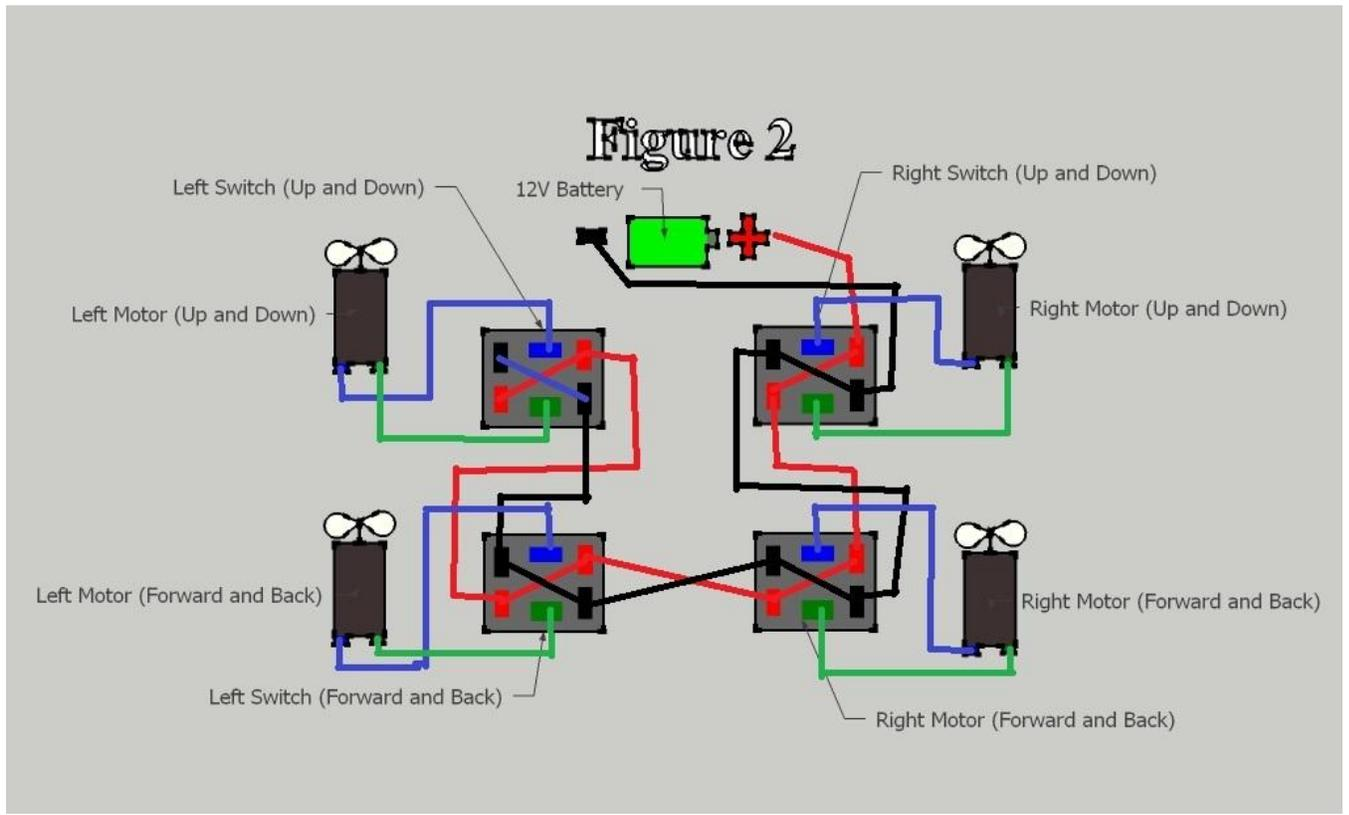
Control Box Wiring Schematic
