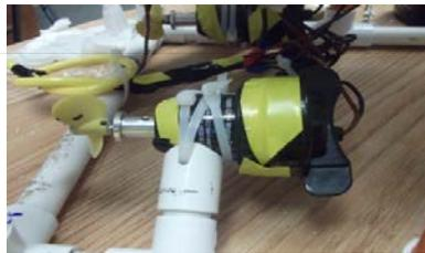
**Figure #8: Johnson Bilge Pump Motor**
