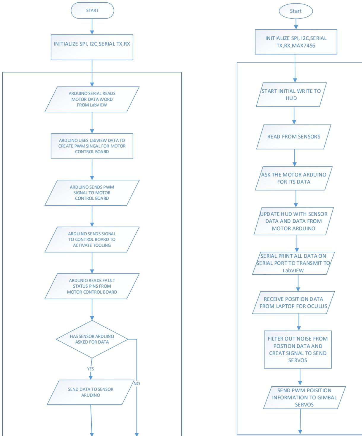
FIGURE 5 FLOWCHART SHOWING THE SOFTWARE FLOW OF THE ARDUINOS. MOTOR ARDUINO ON LEFT, SENSOR ARDUINO ON RIGHT
