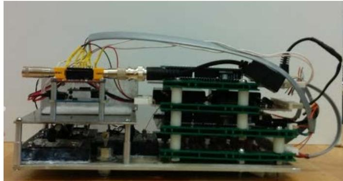
FIGURE 8 THIS PHOTO SHOWS A SIDE VIEW OF THE SHELVING SYSTEM DEVELOPED TO SAVE SPACE INSIDE THE MAIN HOUSING
