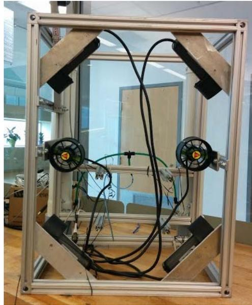
FIGURE 2 THIS PHOTO SHOWS THE VECTOR FORMATION OF THE THRUSTERS AS IT APPEARS FROM THE UNDERSIDE OF THE CRAFT. (HOUSINGS NOT SHOWN)
