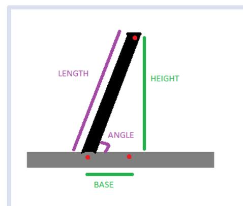
FIGURE 7 ARTIST INTERPRETATION OF THE LASER'S BEING USED TO DETERMINE THE LENGTH AND ANGLE OF THE WELLHEAD. PURPLE INDICATED CALCULATED VALUES, GREEN INDICATED MEASURE VALUES
