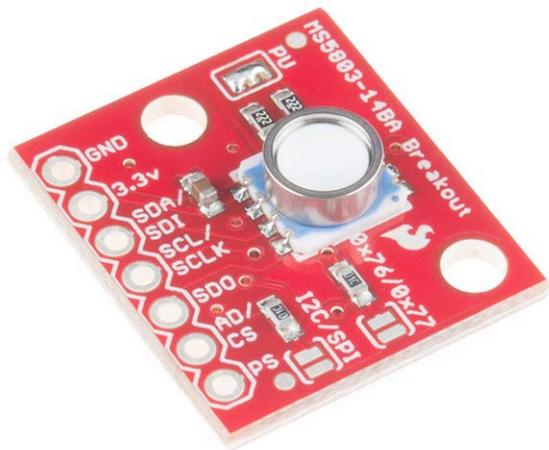
Figure 6: Sparkfun Pressure Sensor
