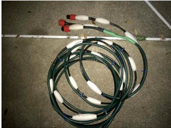
Figure 9: Tether consisting of two cables and gill net floats. (L. Potter)
