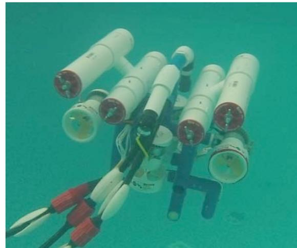
Figure 7: The backside of the FDS 2016 showing the four top ballast tubes that keep the vehicle stable underwater. (L. Potter).
