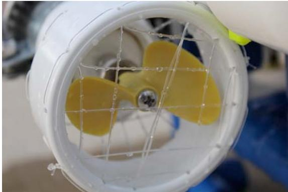
Figure 3: The Kort nozzles with safety netting
