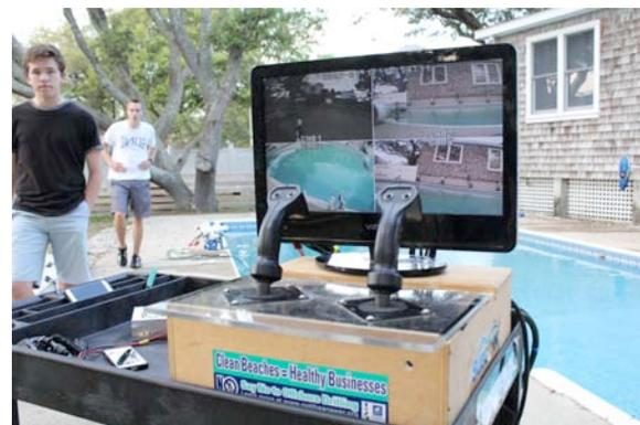
Figure 12: The control box with joysticks (Photo: L. Potter)
