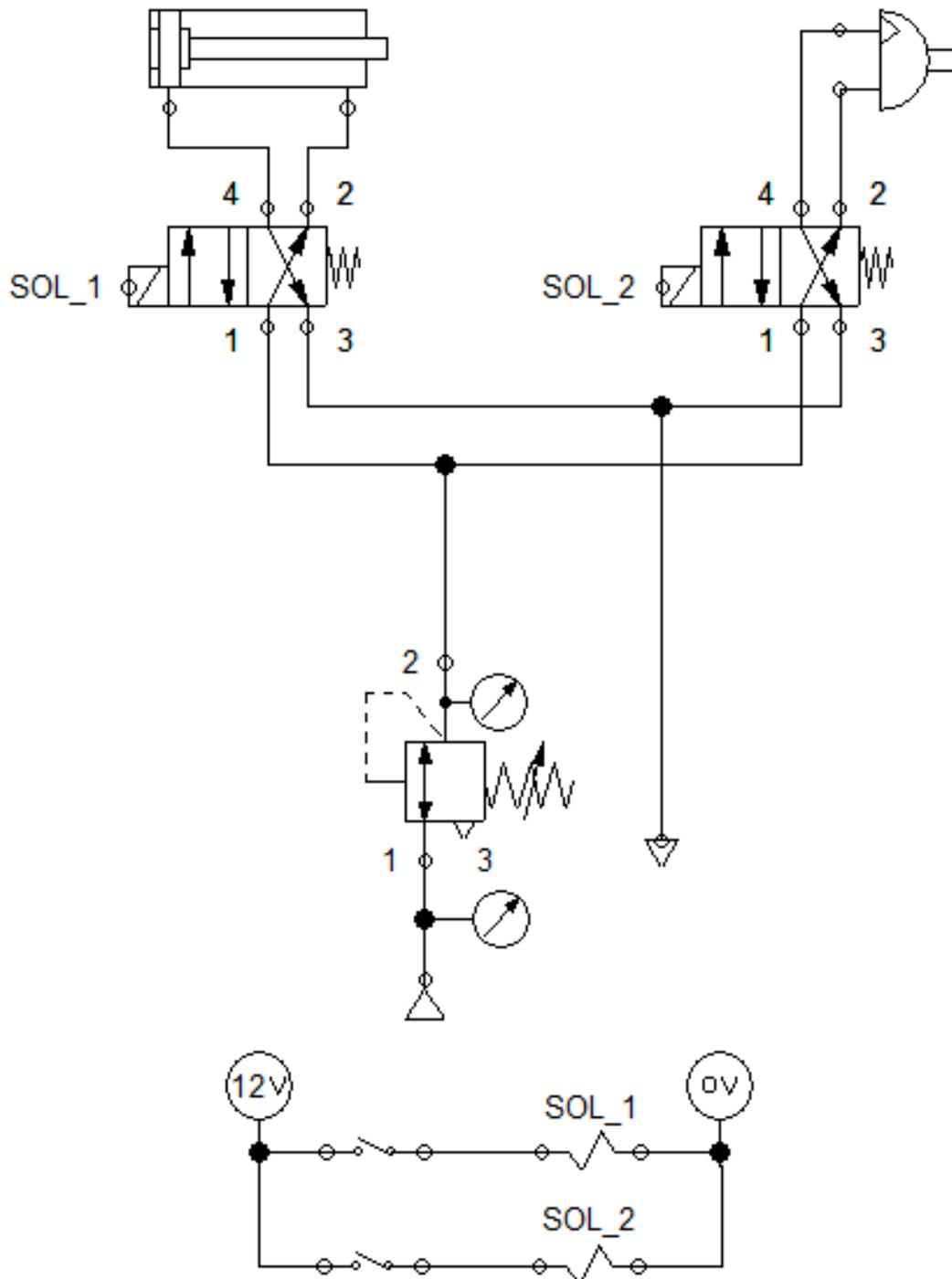
Pneumatics system enabling the claw function of the ROV
