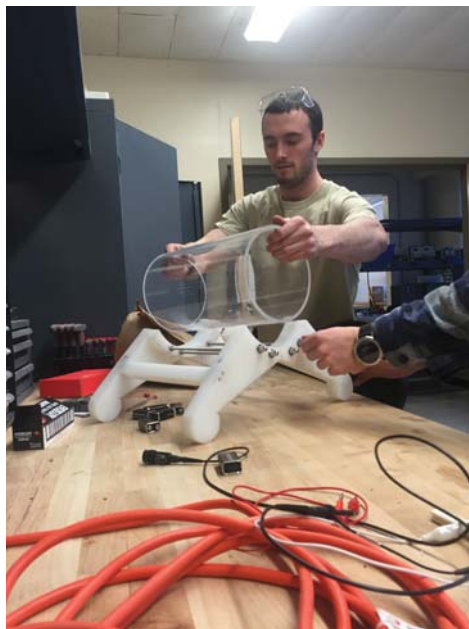
Figure 4: Test fitting the housing on the freshly machined structure
