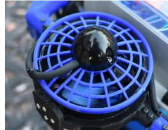
(Left to Right) Three-quarters view of the Argo VI; Neat and deliberate wiring in the onboard electronics enclosure; Shrouded Blue Robotics T100 thruster (Photo Credits C. Barrett)
