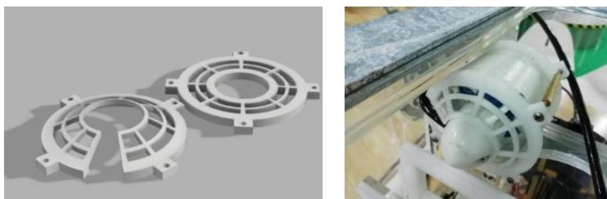
Figure 2.2.3 & 2.2.4: The shield of the propeller
