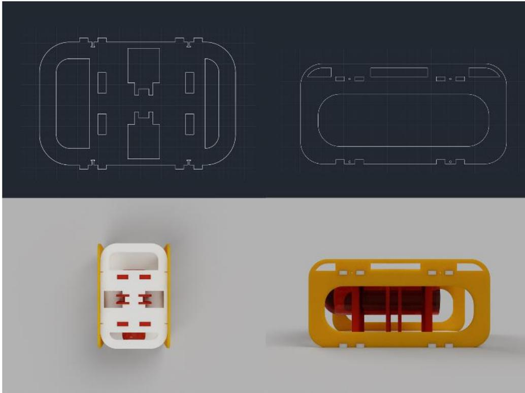
Figure 3.2.2: CAD design and 3D model for side(right) and upper board(left)
