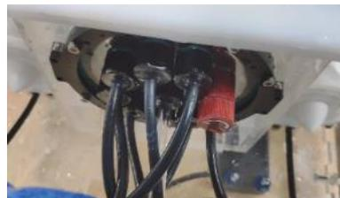
Figure 2.2.2: The tether has strain relief
