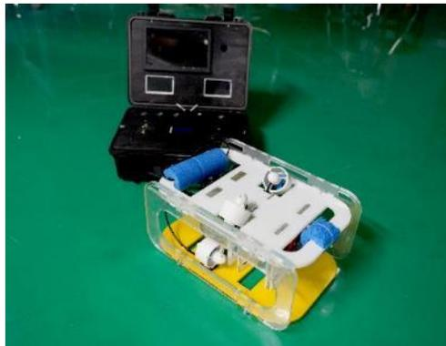
Figure2.3.1: The ROV and the control box
