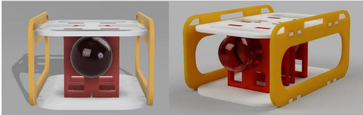
Figure 3.2.1: Rendering of frame with hub attached
