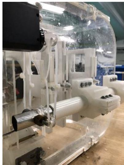
Figure 3.4.1: PVC tube and motor attached to metal arm
