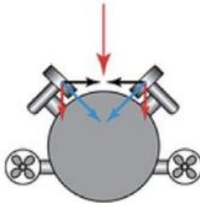
Figure 3.3.2: Illustration of the forces during diving
