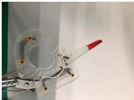
Figure 3.4.4: Mechanical arm claw and hook
