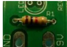
2. With the meter still on DC volts, leave the black meter lead on the GND connection and then place the red meter on each side of the R1 resistor. On one side you should get the battery voltage and on the other side you should get less than the battery voltage, approximately 3V, since the resistor used up or dropped some of the available battery voltage. If you do not get these readings, then most likely there is a poor soldering connection on the resistor. Resolder both sides of the resistor.
