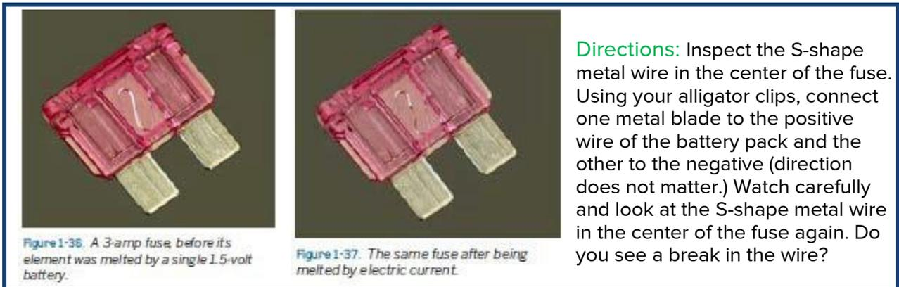
\*Note: If your battery pack is weak it might not blow the fuse, try the 6-volt lantern battery instead.
